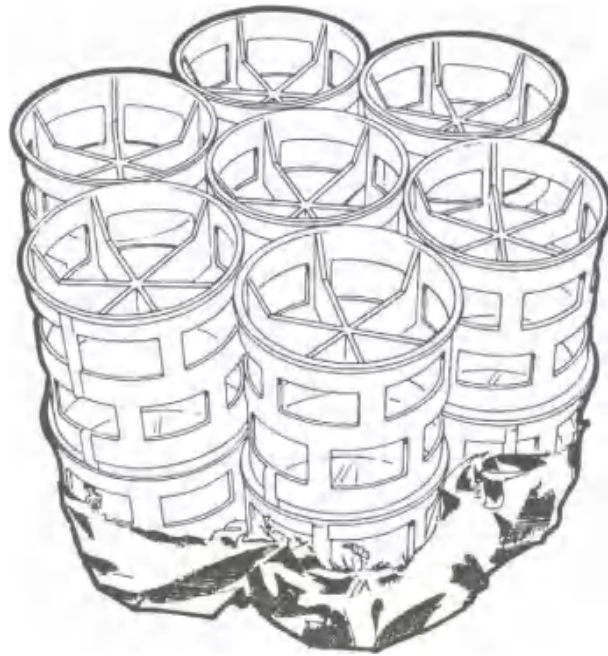
FIGURE 9.8 The UK standard colonization unit used as an artificial substrate for macro-invertebrates in rivers sites not suitable for sampling with either a hand-net or Surber sampler. (Reproduced from Department of the Environment (1983b) with permission of Her Majesty's Stationery Office, London.)
