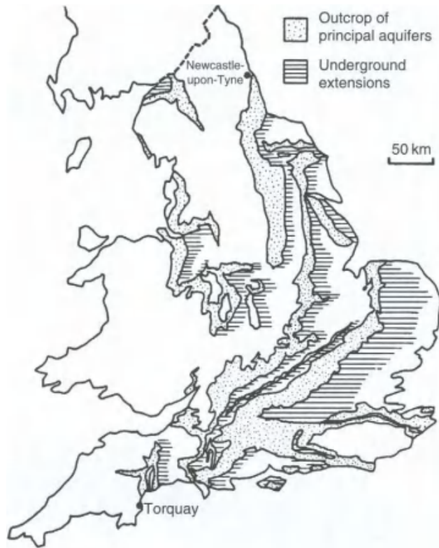
FIGURE 2.3 Location of the principal aquifers in England and Wales. (Reproduced from Open University (1974) with permission of the Open University Press, Milton Keynes.)
