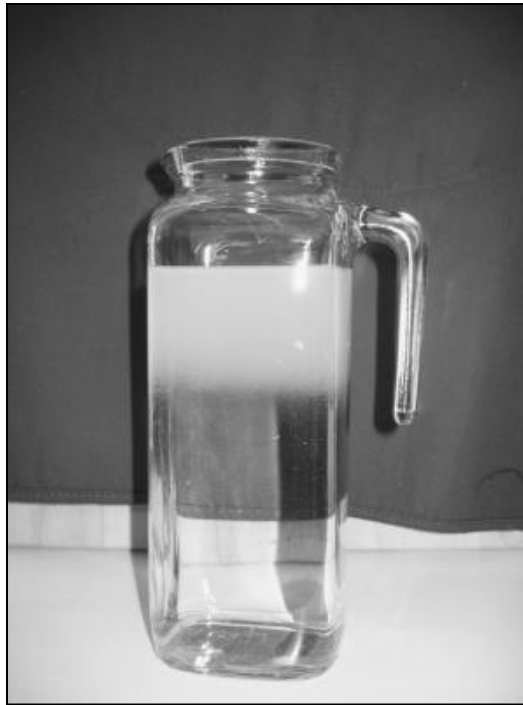
Figure 3-17 Pitcher of water with water supersaturated with air, showing bubble cloud rising toward water surface
