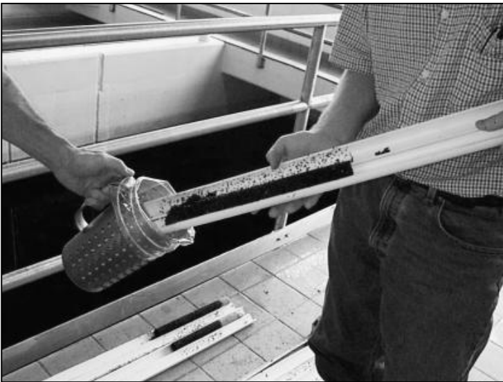
Figure 10-12 Hinged core samplers opened to permit examination of anthracite and sand layers extracted from filter bed
