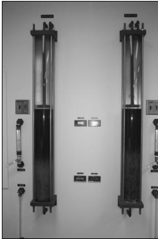
Figure 2-6 Pilot filters used for evaluating coagulation efficacy
