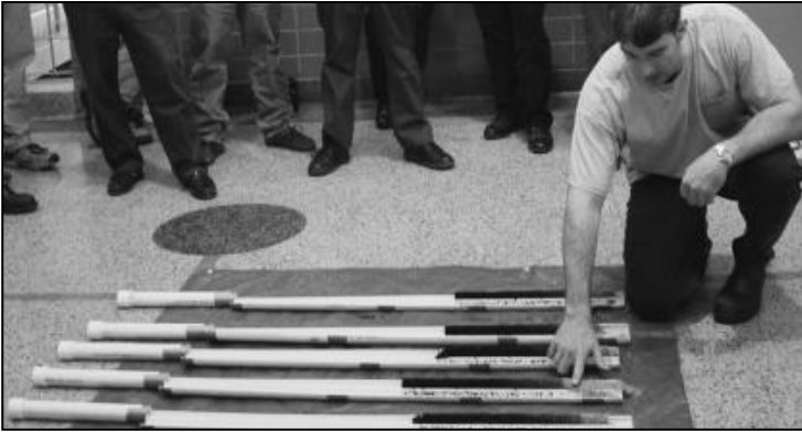
Figure 10-12 Hinged core samplers opened to permit examination of anthracite and sand layers extracted from filter bed
