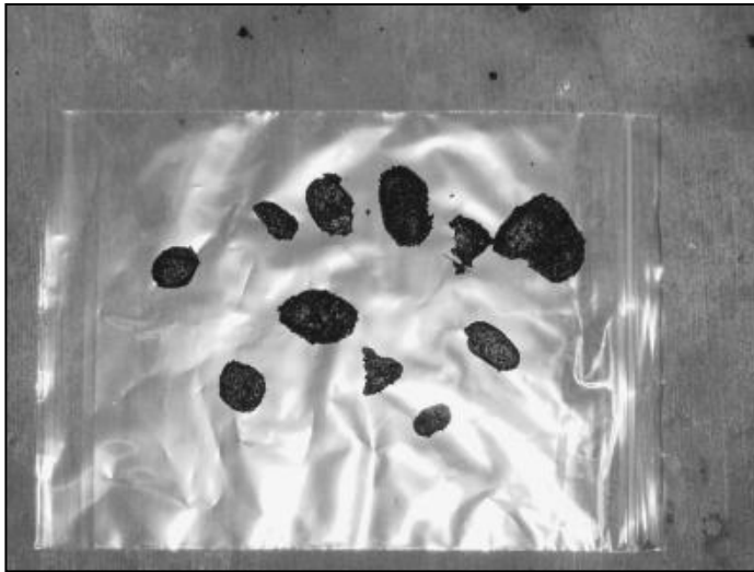
Figure 10-16 Small mudballs removed from a filter
