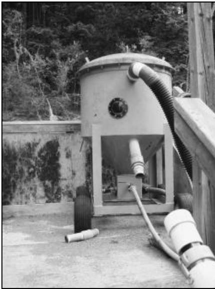
Figure 11-7 Sand washer for cleaning sand before it is replaced in a slow sand filter bed
