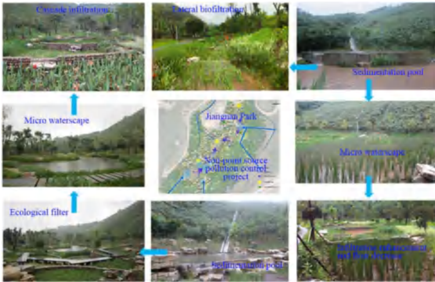
Figure 13.9 Rainwater treatment facilities integrated into a non-point source control system (photos by authors).
