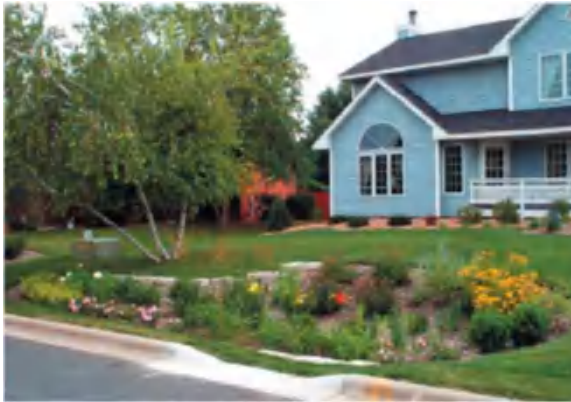
Figure 4.7 Rain garden with curb cut on a residential street (photo by authors).
