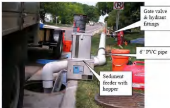
Figure 4.12 Synthetic runoff testing of sediment capture by an underground pre-treatment chamber (source: Erickson et al., 2013 ).
