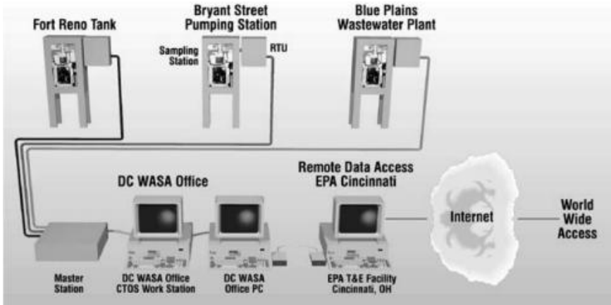
FIGURE 14.3 Relationship between the SCADA system and the transmission of the data through the Internet.
