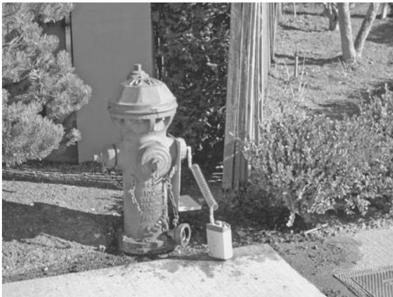
FIGURE B.34 Data logger with internal pressure sensor. (Source: Reinhard Sturm.)
