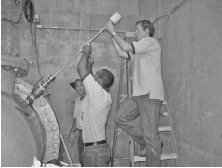
FIGURE B.5 Velocity profiling using a turbine insertion meter. (Source: Reinhard Sturm.)
