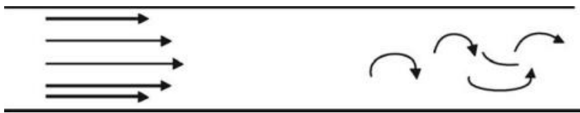
FIGURE 22.3 Difference between laminar and turbulent flow. (Source: Julian Thornton)
