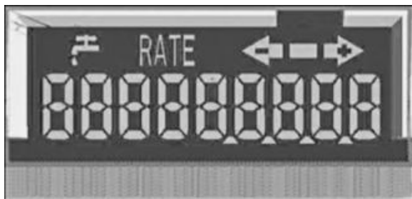
FIGURE 13.13 LCD display of solid state register for Neptune meter capable of detecting reverse flow (backflow) events and leaks on internal plumbing. The arrow indicators show the direction of flow and the faucet indicator reveals the presence of a leak. (Source: Neptune Technology Group.)
