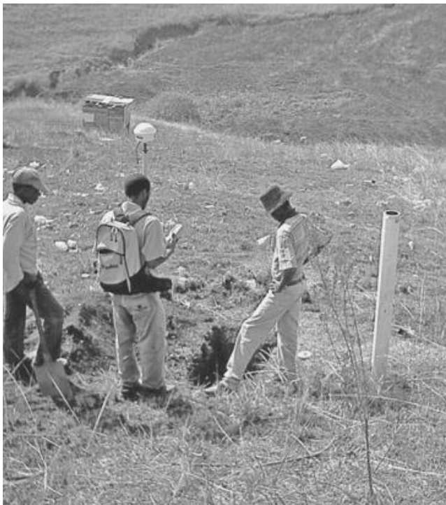
FIGURE 16.2 Using GPS to locate fittings.
