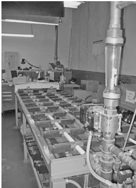
FIGURE 12.8 Water meter test bench for accuracy testing of water meters smaller than 3-in size.
