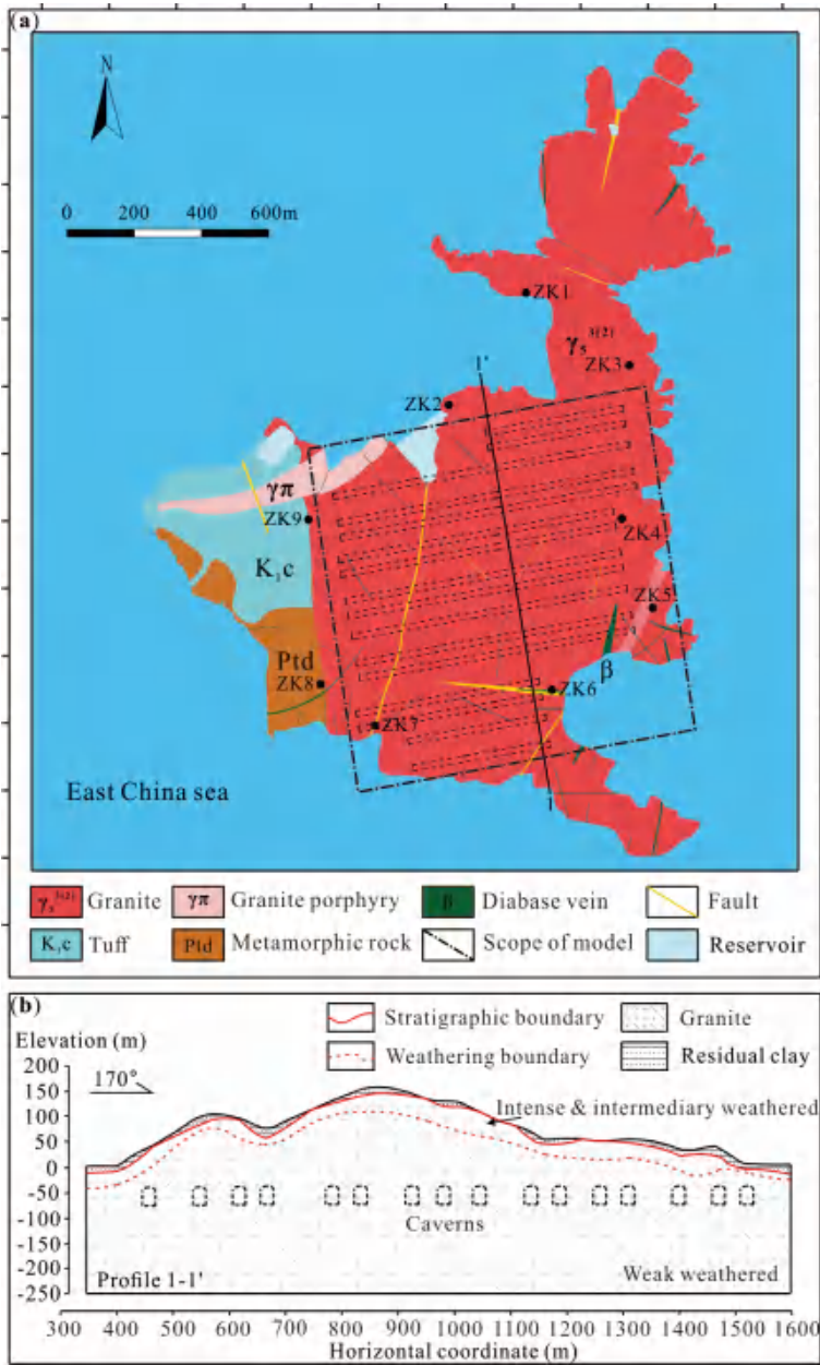
Figure 3. Geological map of the study area: (a) plane map, ZK1-ZK9 are the number of groundwater table monitoring boreholes; (b) profile map.
