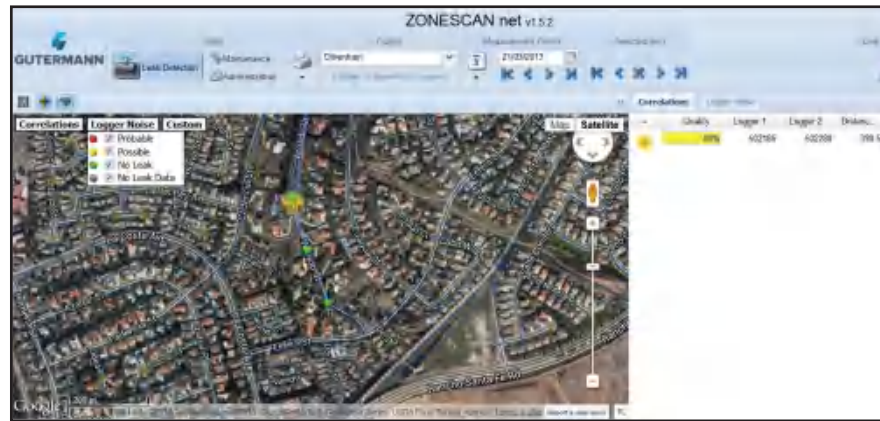
Figure 7-19 Screenshot of the aerial dashboard display of the leak noise transmitter system in use in the Olivenhain Municipal Water District
