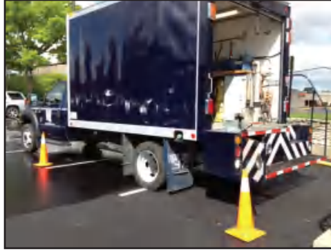
Figure 5-10 Truck equipped with large meter testing apparatus for in-situ meter testing at Louisville Water Company
