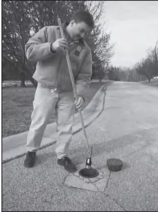
Figure 6-8 Leak noise loggers help to automate the leak survey process and provide consistent sounding capabilities for effective leak detection
