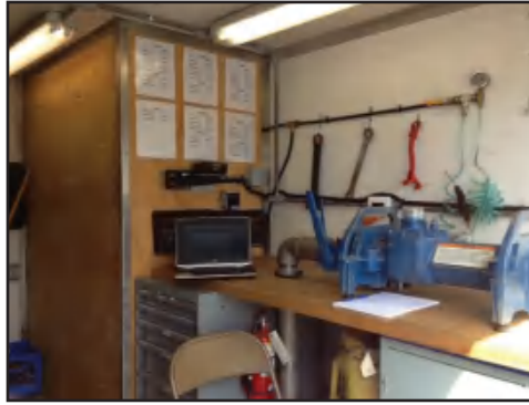
Figure 5-12 Interior of large meter test truck showing calibrated test meter
