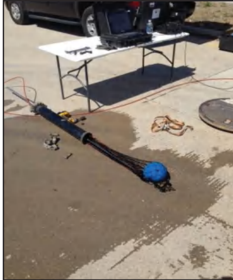
Figure 7-23 Free-flowing leak detection sensor inside the retrieval tool
