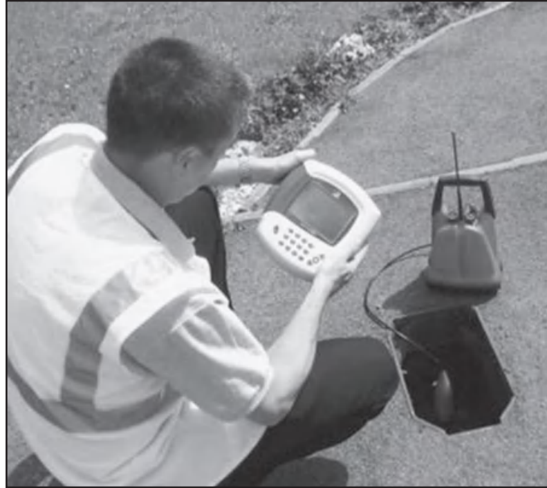
Figure 6-7 Leak correlators have become a standard pinpointing tool of the leak detection squad in many water utilities
