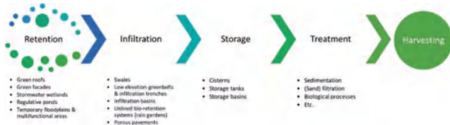
Fig. 3 Scope of features of the LID technologies used for Sponge City implementation
