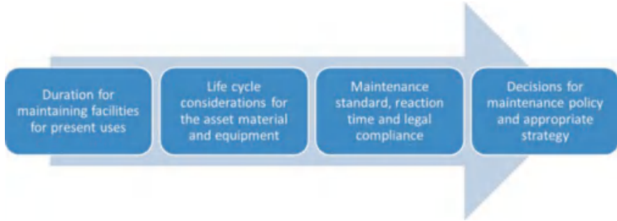
Fig. 17 Proposal for the procedure for defining a maintenance strategy according to specifications of Lee und Scott (2009)
