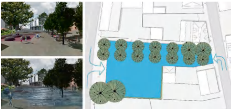
Fig. 16 Multifunctional design of an open space as retention basin for extreme rainfall
