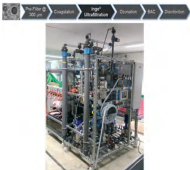
Fig. 13 Inge ultrafiltration pilot plant as part of the integrated treatment scheme for high-quality drinking water production
