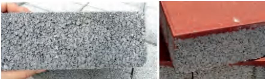
Fig. 4 Examples for pervious pavement materials
