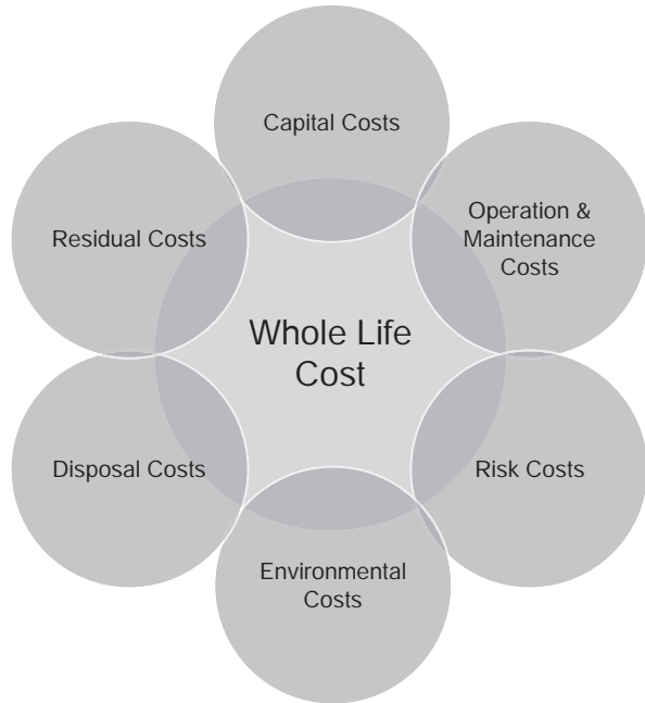
Fig. 4.7 SuDS cost elements considered in a whole life cost (WLC) assessment. (Based on HR Wallingford 2004)
