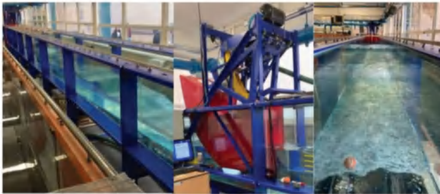
Figure 1. Wave flume apparatus. Example of wave generation along the flume (left), wave generator at the upstream section of the flume (centre), and dissipation beach at the downstream section of the flume (right).
