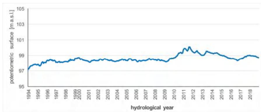
Figure 5. Monthly average potentiometric surface of the Quaternary aquifer in well no. II-22-1 [20].
