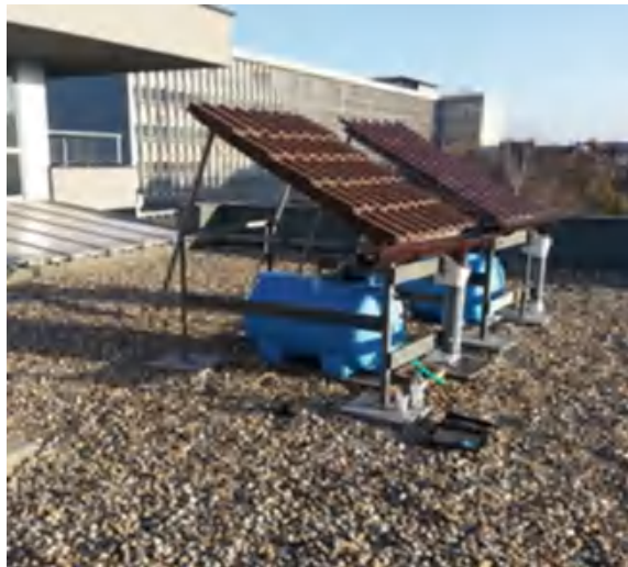
Fig. 30 Location of models on the roof of university library building. Left hand model with ceramic roof tiles, right hand model with organic coated metal roofing (Ahmidat et al. 2013)
