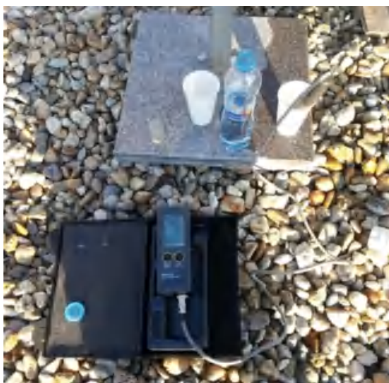
Fig. 32 Analysis of water quality on the spot using multi-parameter water quality sensor HANNA HI 991301
