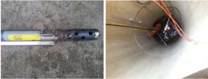
Fig. 25 Multi-parameter water sensor for RHSR quality measurement, type YSI 600 XL, and its location in a concrete shaft
