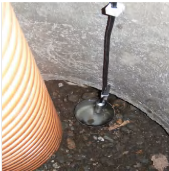
Fig. 12 Pressure sensor for measuring of the water level at the bottom of infiltration shaft (Markovič and Vranayová 2013)
