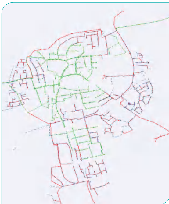
Figure 6.14: The sewer system that is modelled.
