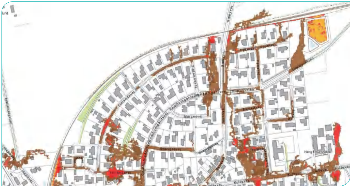
Figure 4.15: Example of a simulation of flooding event in Kalundborg, Denmark. The colors illustrates where there is water on terrain in cm (Brown: 0-10 cm, red: 10-50 cm, yellow: 50-200 cm).
