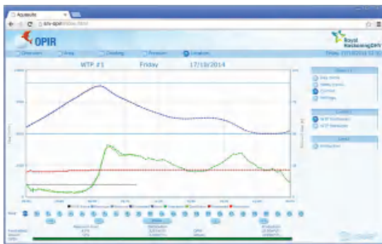
Figure 6.49: User interface, showing trends of forecasted and measured demands, production and transportation flows and reservoir levels.
