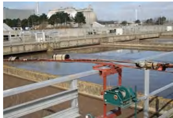
Figure 6.32: Field setup for measuring oxygen concentration profiles.
