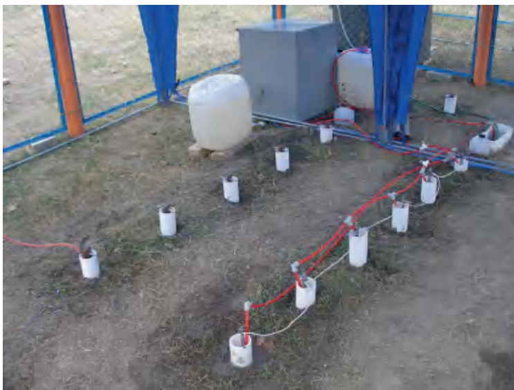
Figure 1. Electrokinetic remediation in-situ
