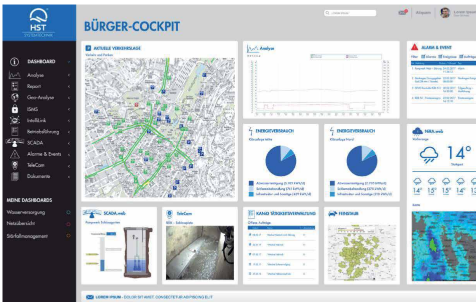
Figure 3. Dashboard KOMMUNAL 4.0 [9] (screenshot shows example for a KOMMUNAL 4.0—cockpit = cockpit of a smart city. It shows different data monitoring systems of water facilities that includes energy consumptions, water level, traffic, dust, alarm events incl. local weather data).
