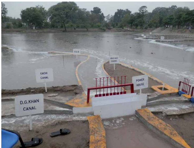
Figure 3. Model Study of Taunsa Hydro Power Project.
