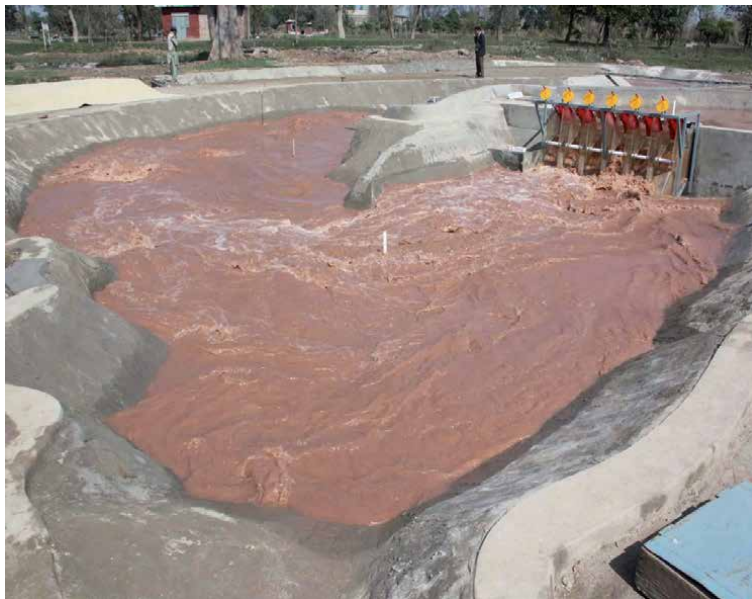
Figure 5. Model Study of Poonch River Sedimentation Project.
