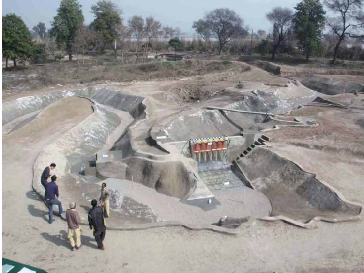
Figure 4. Model Study of Poonch River Sedimentation Project.
