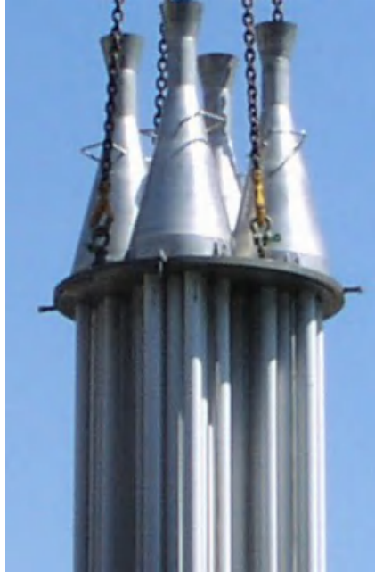
Figure 9 Venturi ejectors installed on the upper clean gas side of the tube sheet.
