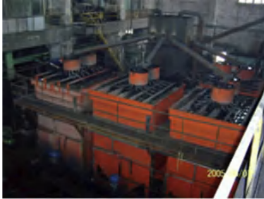
Figure 5 Operation of screen magnetic separators for cleaning of magnetite.
