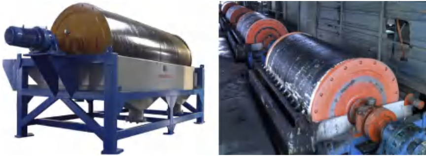
Figure 3 Wet drum magnetic separator (left) and operation for magnetite (right).
