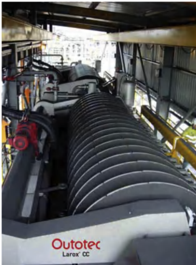
Figure 10 Industrial installation of Outotec Larox CC capillary action filters which have ultrasonic cleaning system ( www.Outotec.com , 2013).
