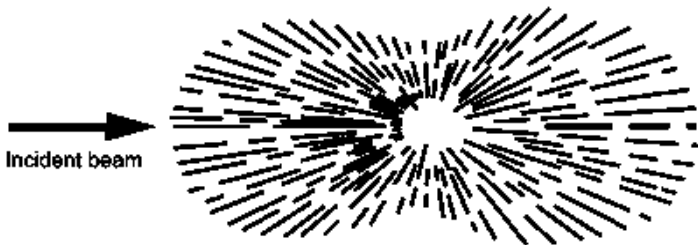
Figure 5 Scattered light pattern for very small particles (smaller than 10% the wavelength of the incident light) (Hach, 1985).
