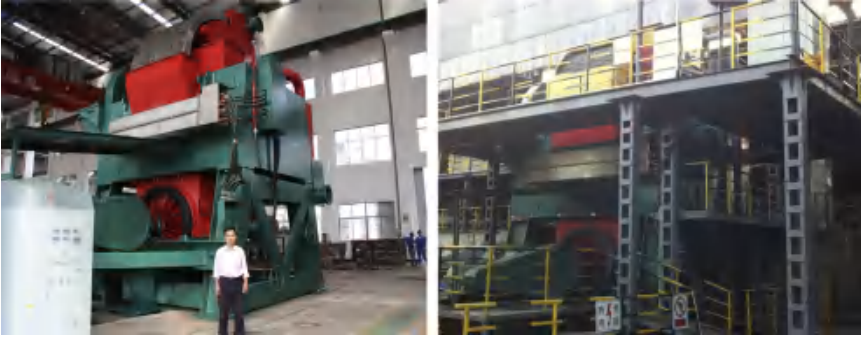
Figure 13 The largest SLon-4000 full-scale pulsating high gradient magnetic separator (left) and operation for concentration of fine ilmenite from tailings (right).
