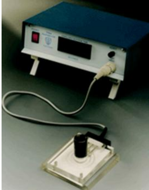
Figure 2 The standard type 304 CST apparatus manufactured by Triton Electronics Ltd, Dunmow, Essex, UK. CST, capillary suction time. Reproduced with permission.
