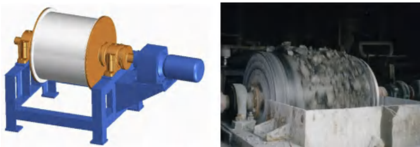
Figure 6 High-intensity magnetic pulley (left) and operation for preconcentration of low-grade magnetic ore (right).
