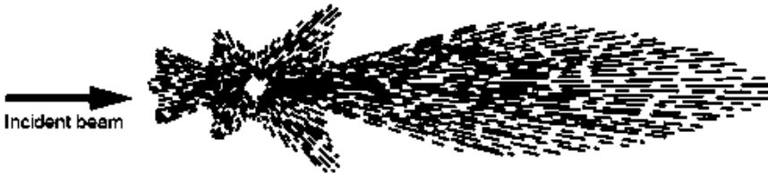
Figure 7 Scattered light pattern for larger particles (larger than the wavelength of the incident light) (Hach, 1985).
