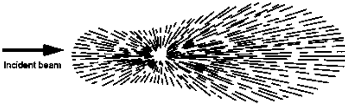
Figure 6 Scattered light pattern for large particles (approximately 25% of the wavelength of the incident light) (Hach, 1985).
