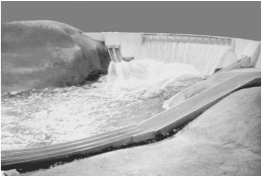
Figure 3.1 Laboratory model of a dam spillway.
