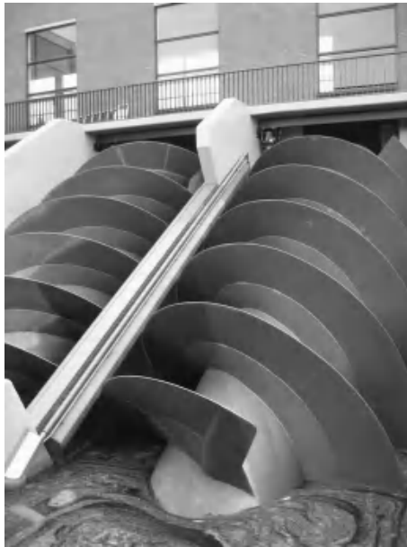
Figure 8.3 Archimedean screw pumps in Kinderdijk, The Netherlands.
