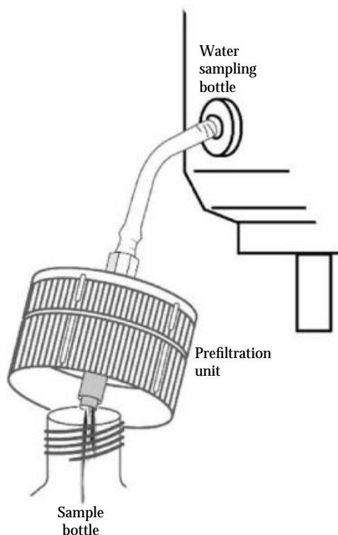
FIGURE 8.3 Prefiltration system fitted to the water sampling bottle (Niskin or Go-Flo bottle).
