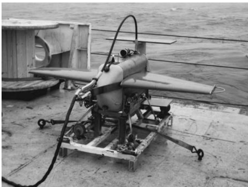
FIGURE 1.5 The towed instrument SeaSoar modified to an online sampling platform. (Photo kindly provided by Dr. Burke Hales, Oregon State University.)
