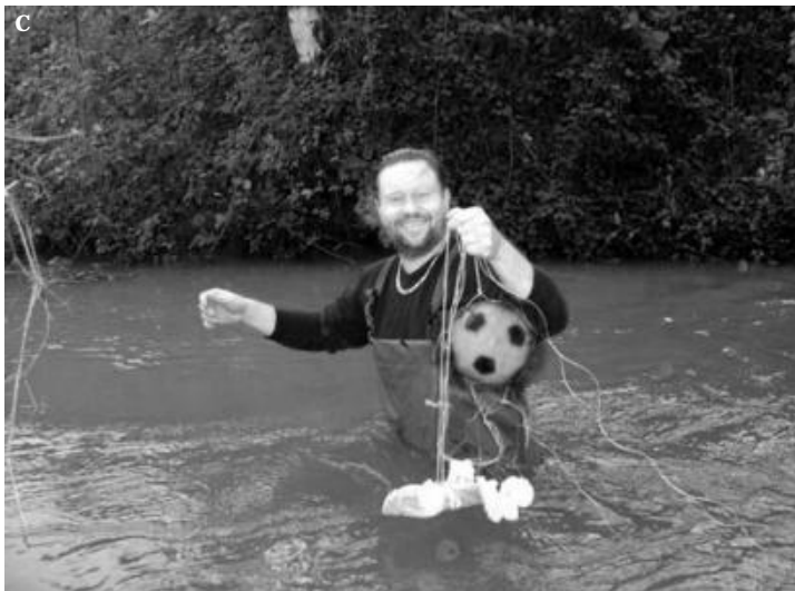
FIGURE 16.1 The POCIS device and its application to pharmaceutical analysis in river and estuarine waters. (A) Component parts of a POCIS, (B) assembled sampling devices, and (C) use of sampler devices in river and estuarine waters.
