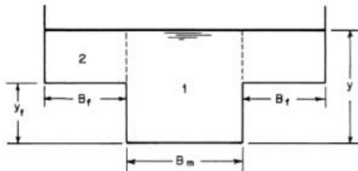
Fig. 3-8. Compound channel cross section
