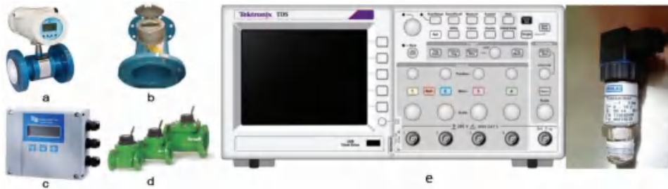
Figure 2. Equipment to measure flow (electromagnetic: (a,c), propeller volumetric: (b,d)) and pressure around the cross-junction (oscilloscope and pressure transducer: (e)).
