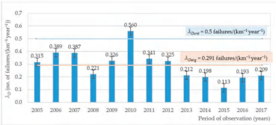
Figure 4. The failure rate for distribution pipes over the distinguished 2005–2017 period.
