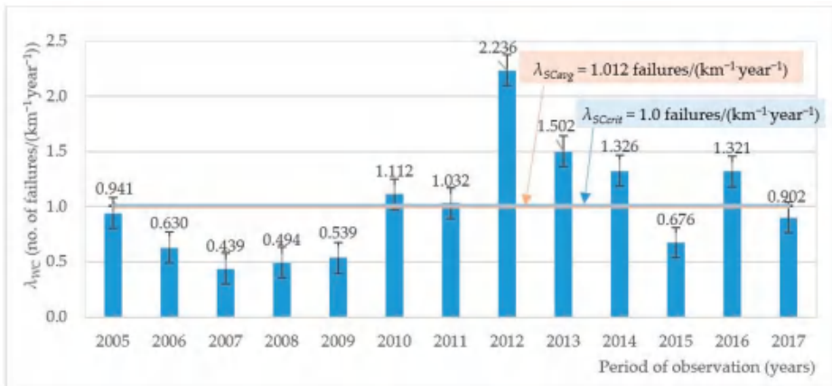
Figure 5. The failure rate for SCs over the distinguished 2005–2017 period.
