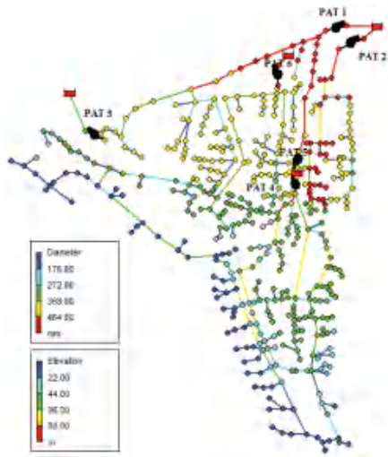
Figure 12. Balerma Irrigation network and PATs location.
