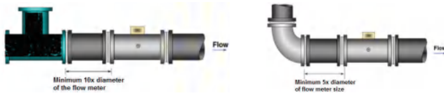
Figure 5. Installation requirements for different pipe layouts.
