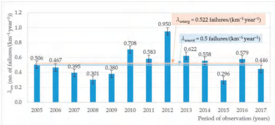
Figure 2. The failure rate for the whole network over the distinguished 2005–2017 time period.
