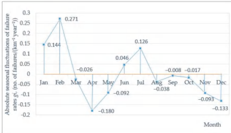
Figure 8. Absolute seasonal fluctuations of failure rates in WDN, in (no. of failures/(km -1 .year -1 )).
