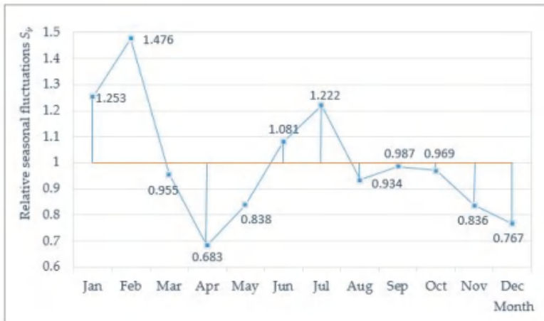
Figure 7. Relative seasonal fluctuations of failure rates in WDN.
