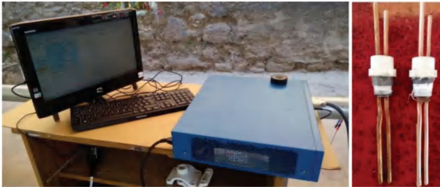
Figure 4. Equipment for stimulus-response technique.
