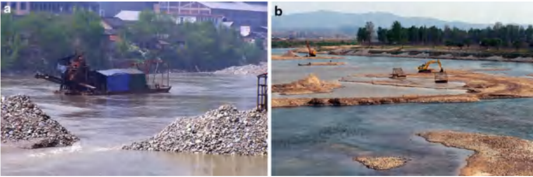
Fig. 3.19. (a) Gold placer mining in the Bailong River, a tributary of the Jialing River in Sichuan; (b) Gravel mining for building materials from the Qingjiang River, a tributary of the Yangtze River.
