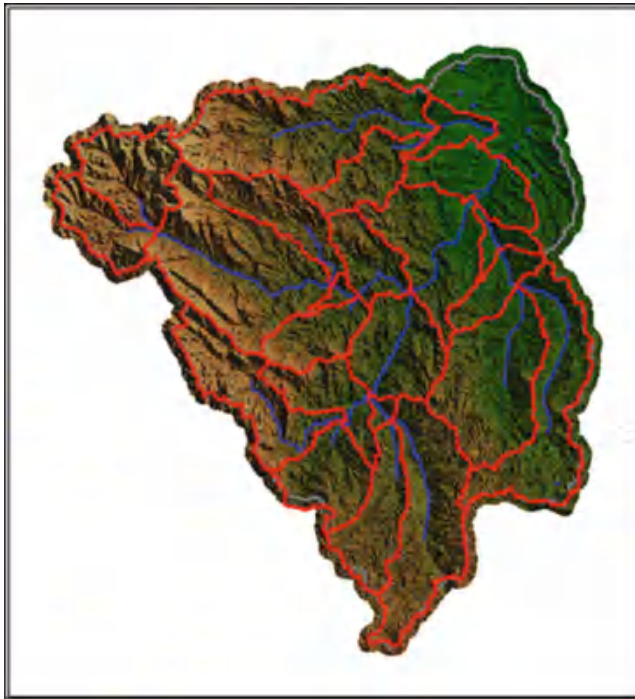
Fig. 7.4. DEM processing routines are applied to extract stream networks and watershed.
