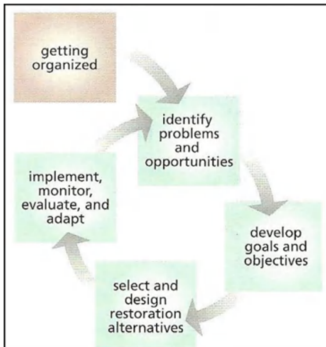
Fig. 4.10. Planning process of river restoration work (cited from the figure on p. II-ii in the literature [4]).
