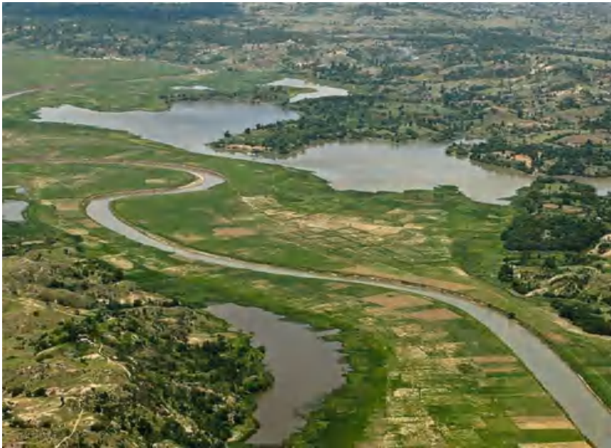
Fig. 5.5. Photograph of deposits in Peligre reservoir during seasonal drawdown for power production (photo: G. Morris).
