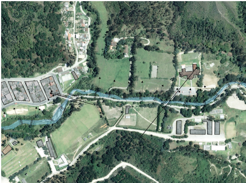
Figure 2.37 Flooding sheet resulting in the neighborhood of the Zamora Huayco district and previous section
