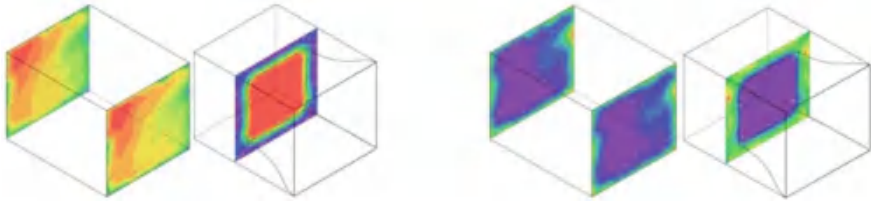
Fig. 11.5 Experiment: Diagram of velocity field distribution (left) and turbulence intensity (right) when passing through the space without cross-sectional change and in the outflow from the narrowed space [23]
