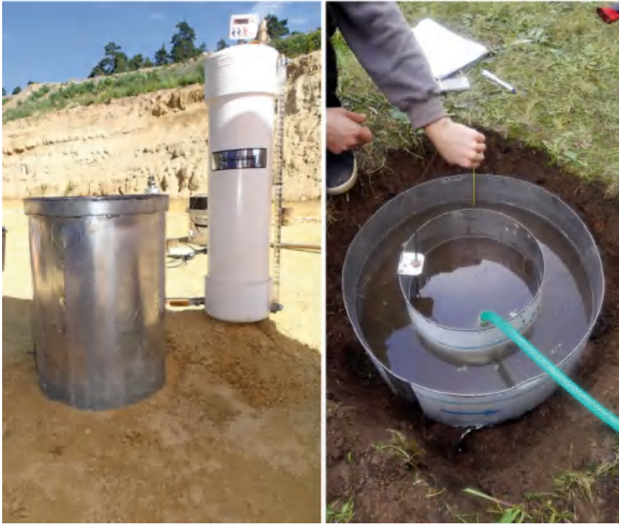
Fig. 4.14 Infiltration test using an infiltration cylinder
