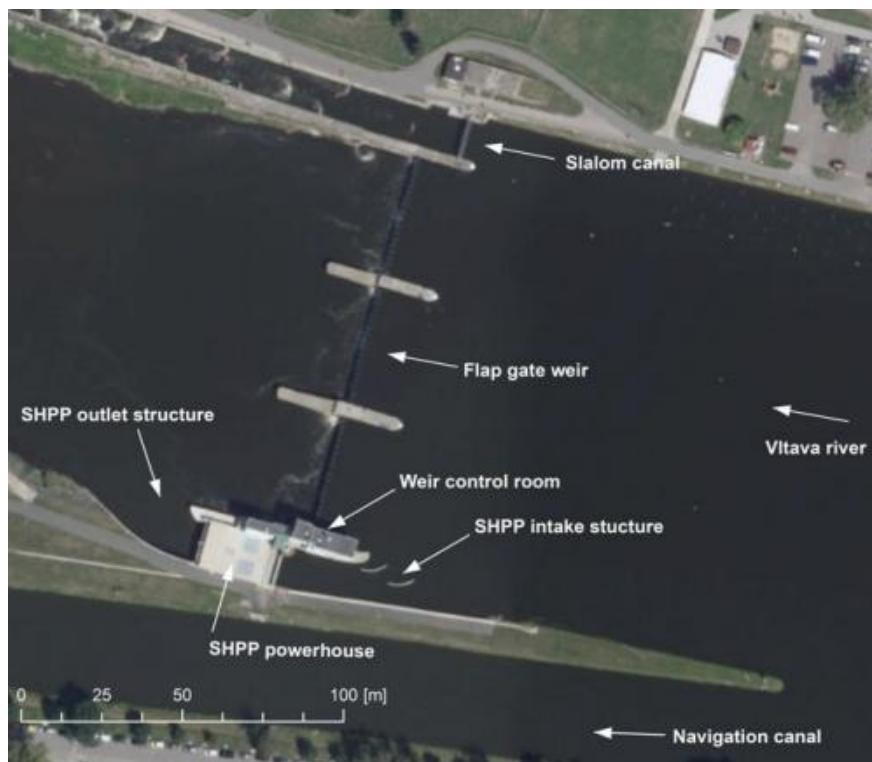
Fig. 15.25 Situation of SHPP Troja (based on data [10])
