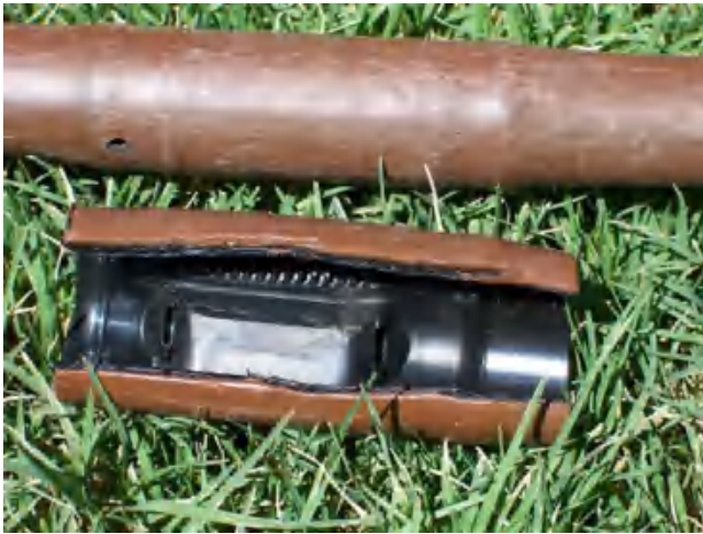
Fig. 15.6 Inline drip tubing
