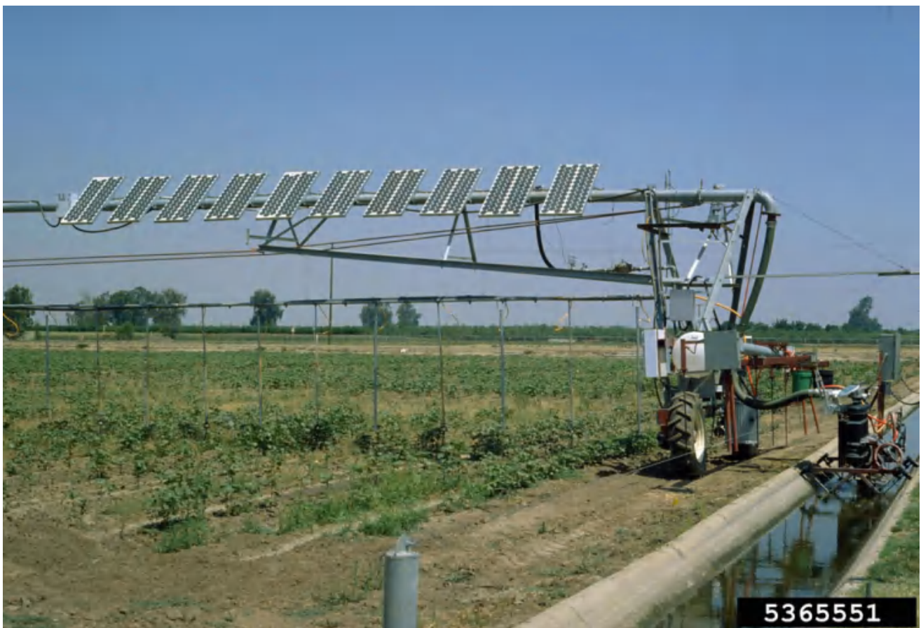
Fig. 1.8 A canal-sourced linear-move irrigation system in use on a field in Colorado (Credit: GE Cardon, Bugwood.org)
