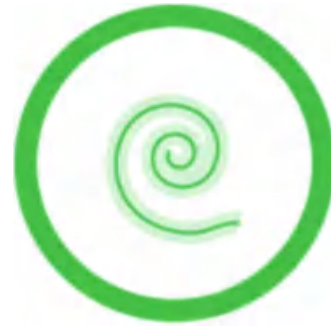
Fig. 15.8 Coil of inline drip tubing around tree
