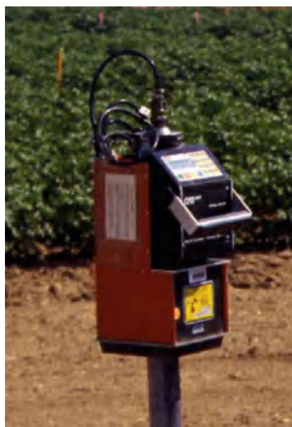
Fig. 3.14 Neutron probe and access tube (Credit Paul Colaizzi, USDA-ARS)
