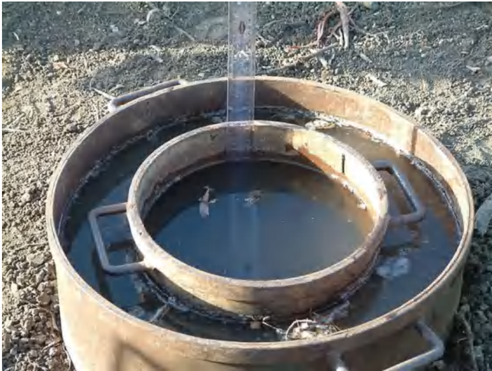
Fig. 20.8 Double ring infiltrometer
