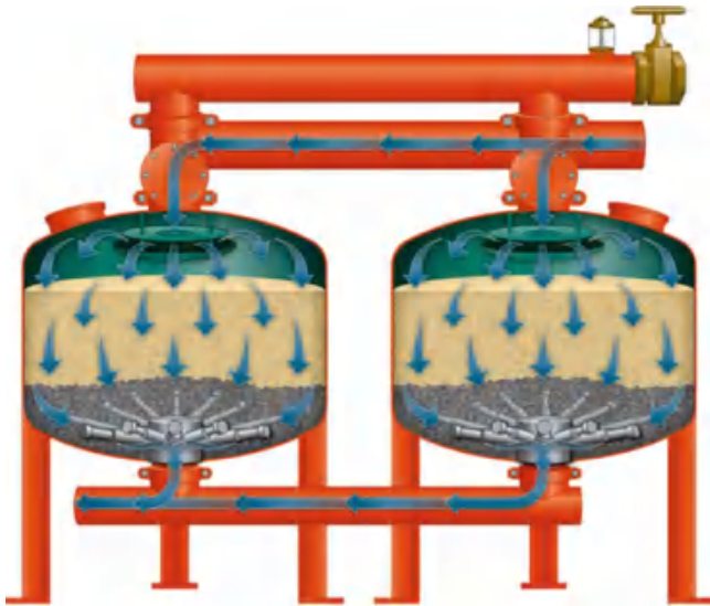
Fig. 17.5 Sand media filters (Credit Yardney Corp)
