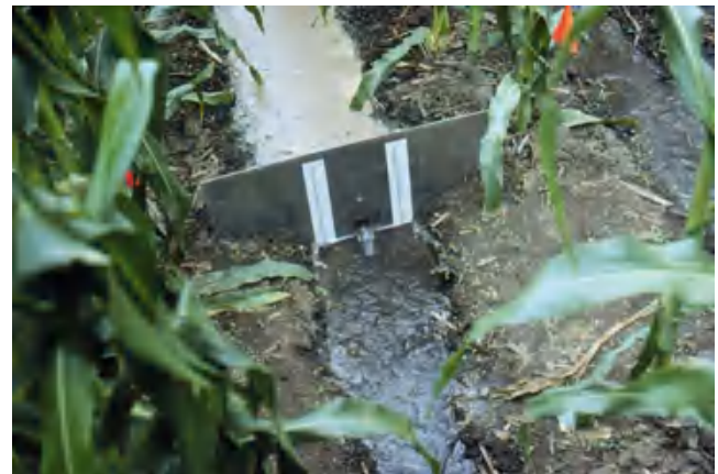
Fig. 20.12 Blocked furrow infiltrometer (Credit NRCS)
