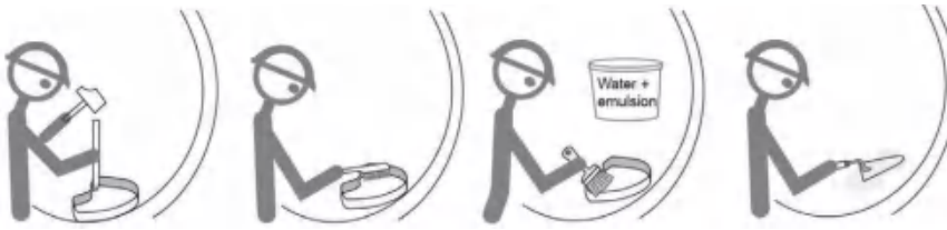
Figure 6.71 Repair of internal cement lining
