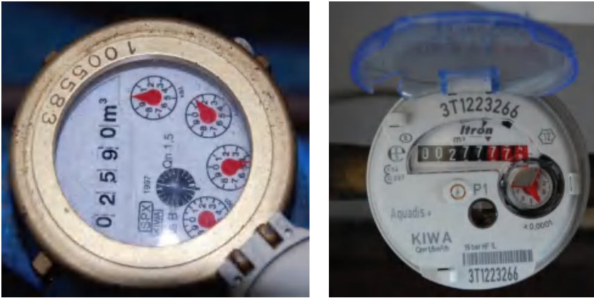
Figure 4.96 Household water meters used in the Netherlands: multi-jet, older type (left-hand side) and single-jet, newer type (right-hand side)
