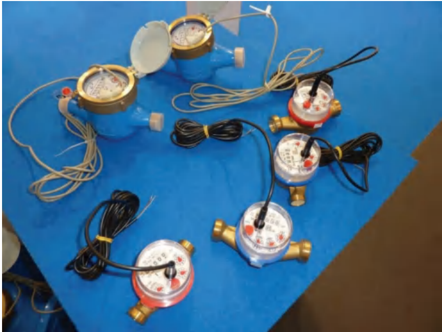
Figure 4.99 Remote reading of water meters
