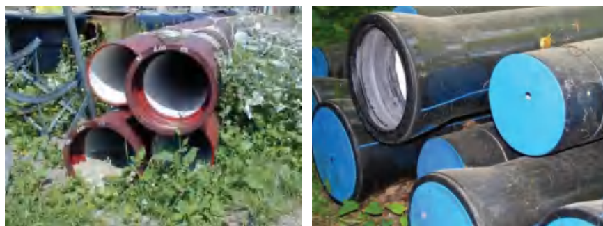
Figure 6.60 Cement-lined DI pipes with (left) epoxy and (right) PE external coatings
