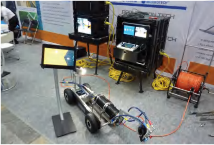
Figure 6.75 Equipment for cement relining of pipes
