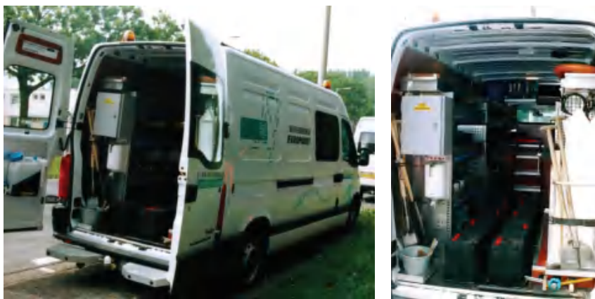
Figure 6.86 Mobile workshop for a quick repair service
