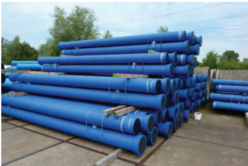
Figure 4.39 Storage of DI pipes
