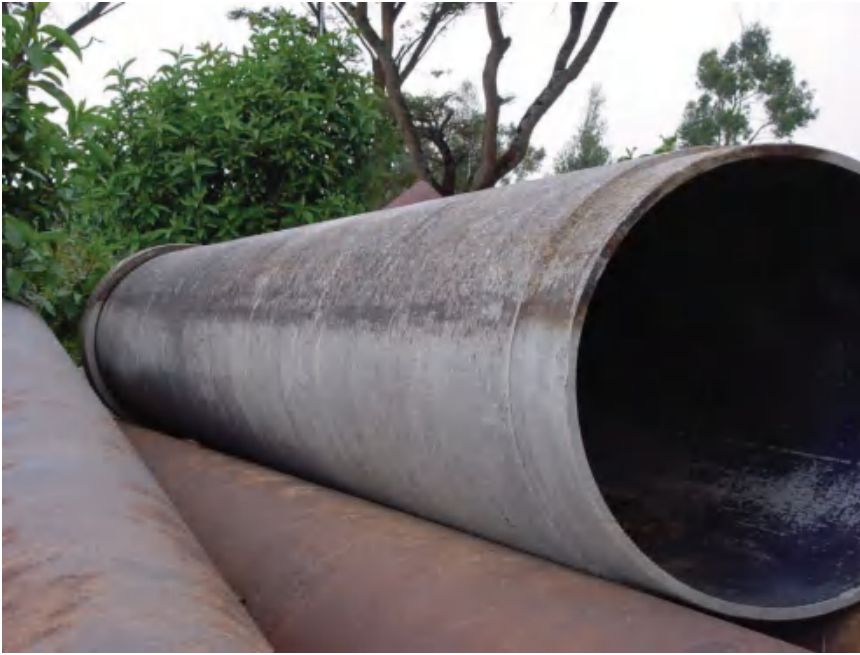
Figure 4.47 Asbestos cement (AC) pipes
