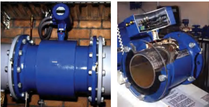
Figure 4.90. Magnetic flow meters
