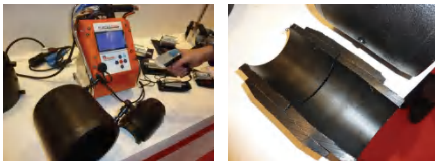
Figure 4.64 Electrofusion equipment (left-hand side: the control box and coupling, right-hand side: the joint)
