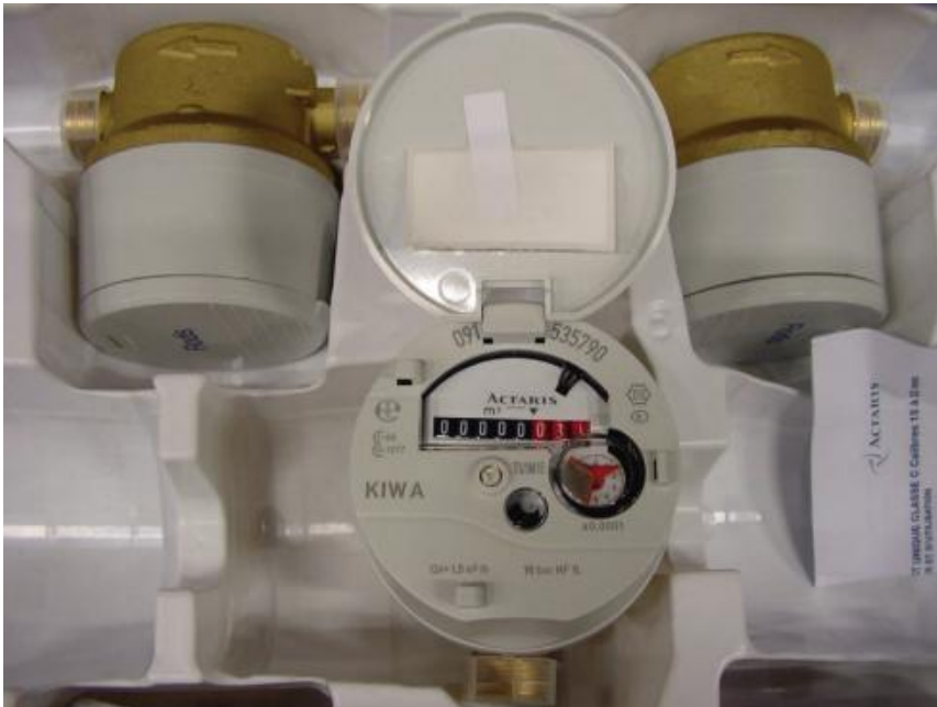
Figure 4.123 A KIWA-certified household water meter with the rated pressure of 16 bar (160 mwc), D = 15 mm and nominal flow Q_n = 1.5 m 3 /h, produced in 2009
