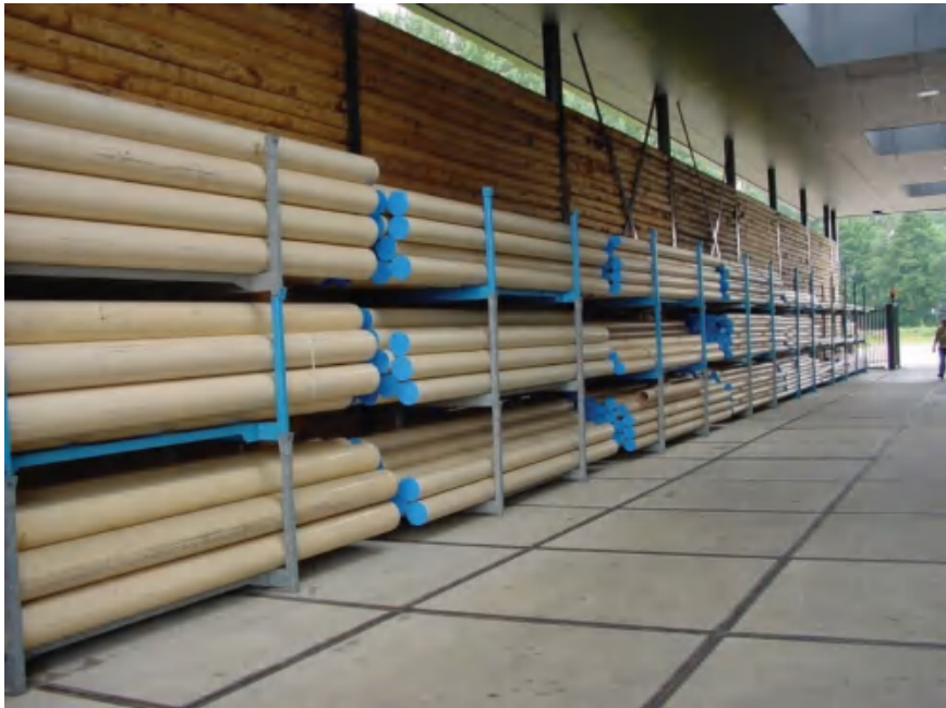
Figure 4.54 Typical PVC pipes used for distribution of drinking water in the Netherlands
