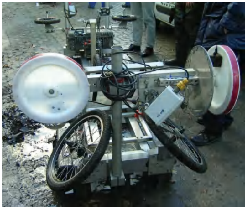
Figure 6.78 Ultrasonic equipment for inspecting the cement lining of reinforced concrete pipes
