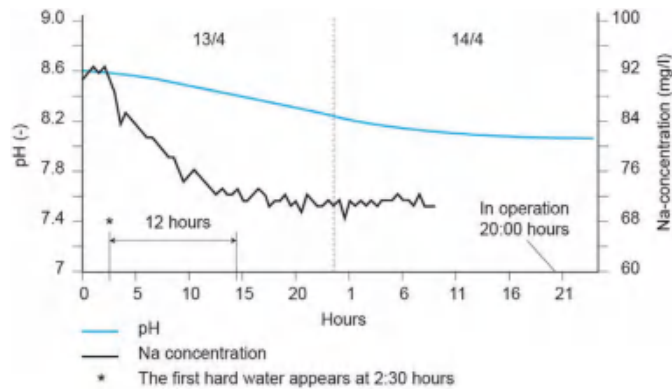
Figure 6.11 Comparison between Na concentration and pH values in the system
