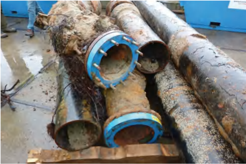
Figure 4.58 Old scrapped CI pipes collected for recycling
