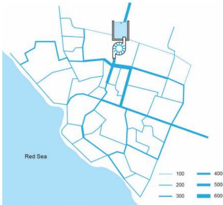
Figure 1.10 The distribution system in Hodaidah, Yemen
