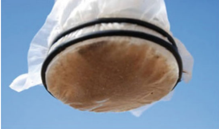
Fig. 3.25 View of the malleable disk base (From Moret-Fernández et al. 2013, reprinted with permission)
