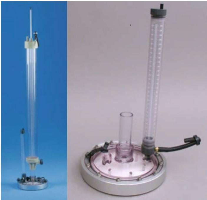
Fig. 3.3 Guelph Tension Infiltrmeter with assembled baseplate unit (From Soilmoisture Equipment Corp. 2008b, reprinted with permission)
