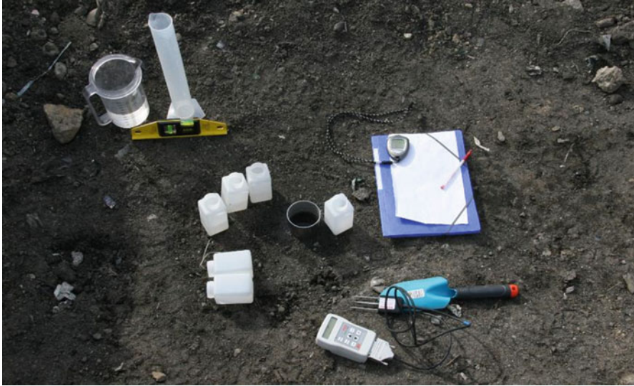
Fig. 3.31 Beerkan experiment apparatus: spirit level to prepare the soil, ring inserted into the ground, prepared volumes of water to be infiltrated, timer and notebook, water content probe
