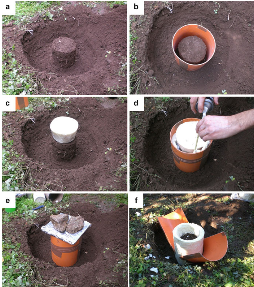
Fig. 2.41 Steps of the realization of a casing in polyurethane foam for applying the SFH technique: (a) exposition of the soil column; (b) placement of the PVC cylinder with opened extremities around the soil column; (c) placement of a stopper in polyurethane foam on the surface of the column; (d) filling of the space between the PVC cylinder and the soil column with polyurethane foam; (e) placement of a tablet and a small weight on the upper end of the PVC cylinder; and (f) detachment of the PVC cylinder from the casing (From Bagarello et al. 2009b)
