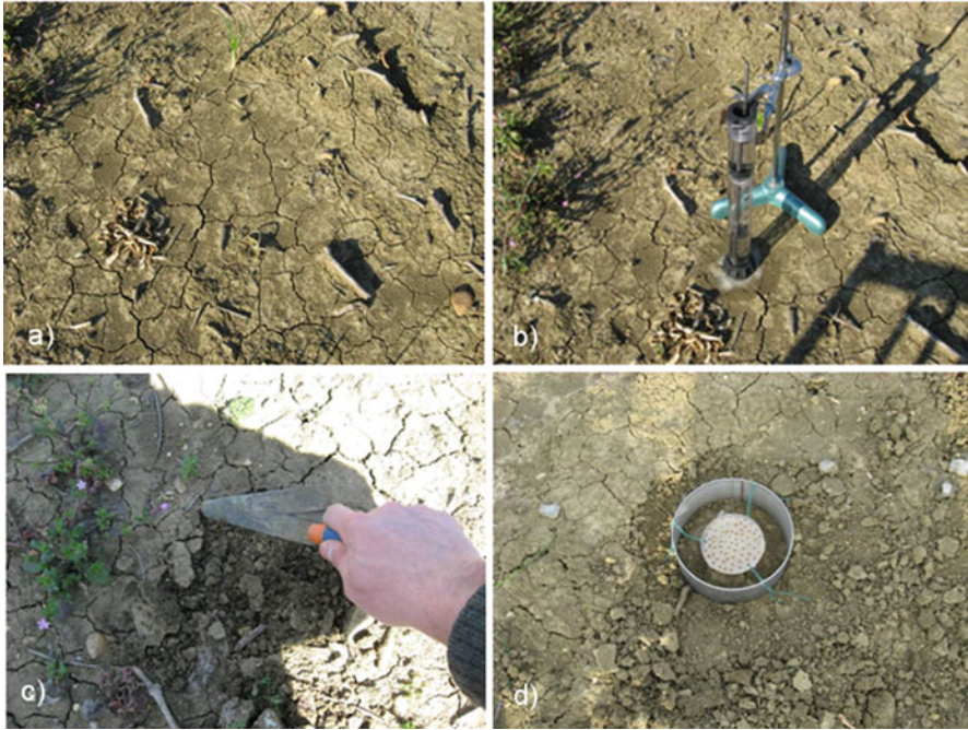
Fig. 4.9 Experimental procedure for determining the hydraulic resistance of the surface soil crust: (a) surface crust; (b) mini disk infiltrometer experiment; (c) crust removal; (d) ring infiltration test (From Alagna et al. 2013)
