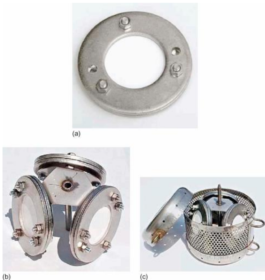
FIGURE 1 (a) A single POCIS, (b) three POCIS assembled together, and (c) the final setup for POCIS before deployment in the field. (From http://www.est-lab.com/pocis.php , with permission)
