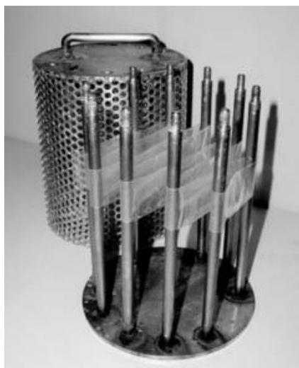
A length of sealed lay-flat PE tubing (the membrane) containing a small volume of triolein (the absorbant phase) is woven around a stainless steel frame
