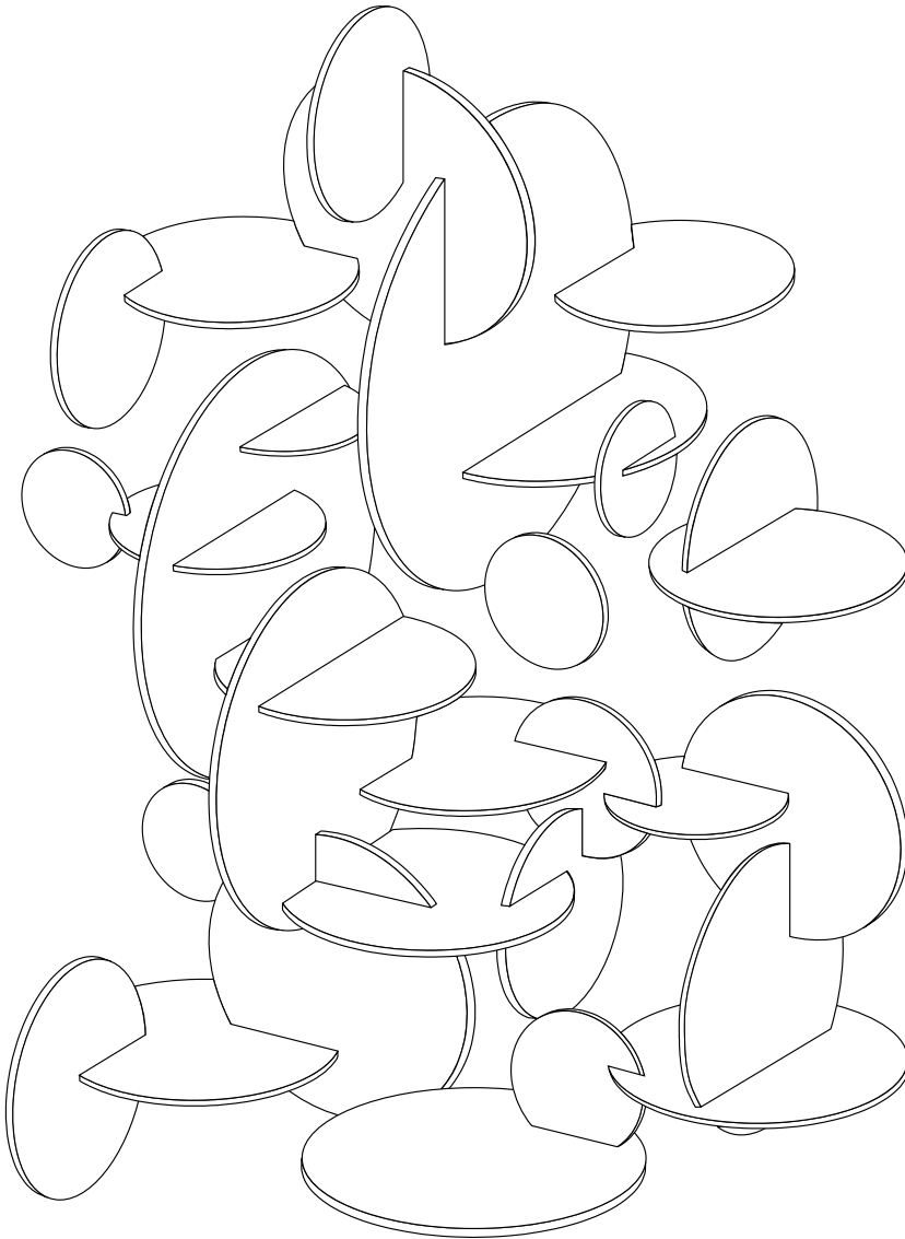
FIGURE 20.28 Three-dimensional conceptual model of disc-shaped fractures that are of random size and oriented orthogonally. (From Long, J.C.S., Gilmour, P., and Witherspoon, P.A., 1985. Water Resour. Res. 21(8): 1105–1115.)
