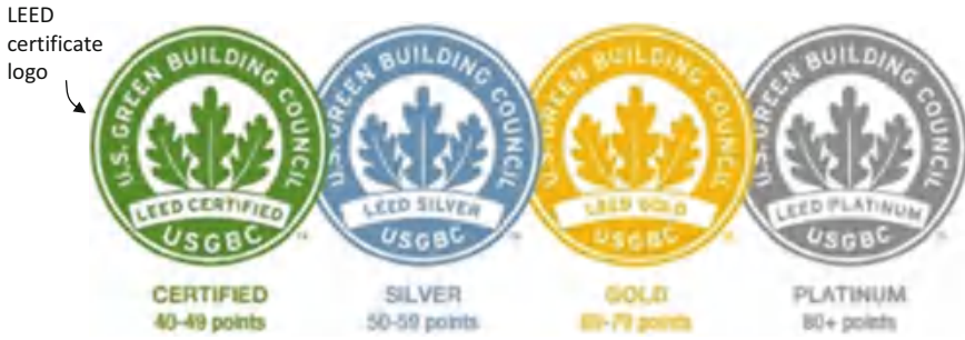
Fig. 14.23 LEED certificate's logo; classification of building sustainability is based on awarded total point score out of maximum 110 points ( www.usgbc.org )
