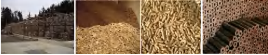
Fig. 2.20 Solid wood biomass fuels in form of grafted wood, woodchips, pellets and briquettes (from left to right; Malamateinios et al. 2017)
