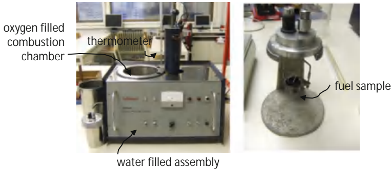
Fig. 2.15 LCV and GCV calorific values of fuel could be determined experimentally by burning a small amount of the fuel in oxygen atmosphere using a “bomb calorimeter”
