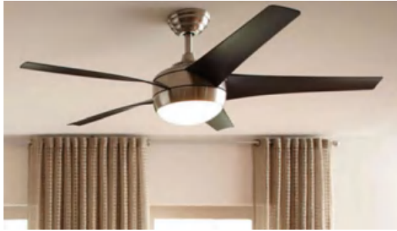
Fig. 1.7 During the cooling season, a ceiling fan blows air downwards and because of higher air velocity residents perceive lower indoor temperature (at 1 m/s a decrease of \approx 3\text{ }^{\circ}\text{C} ); if the tilt of the blades is changed during the heating season, the fan draws air up and reduces temperature stratification without the feeling of an unpleasant draught ( www.powerhousefan.com )
