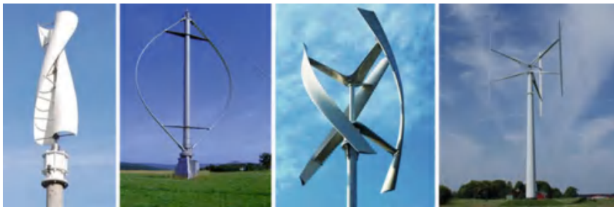
Fig. 7.25 Vertical axe wind turbines (VAWT) for near-by electricity production: Savonius rotor, Darrieus rotor, helical rotor and H-type rotor
