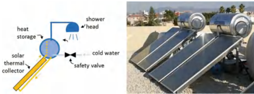
Fig. 10.11 Thermo-syphon DHW solar heating systems (SOLARGE 2004)
