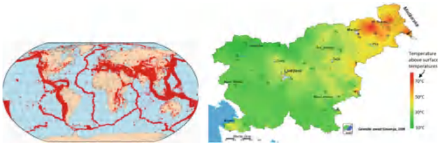
Fig. 2.11 Areas along boundaries of tectonic plates have the largest geothermal potential (left; Ragheb 2017); temperatures 1 km beneath the surface on Slovenian territory indicate significant geothermal potential in the north-eastern region (right) (Geothermal potential in Slovenia, Geološki zavod Slovenije, 2008)
