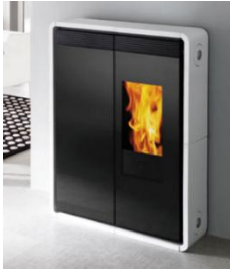
Fig. 6.3 Pellet stove; small storage for pellets (20 kg) is integrated in the stove to enable operation for a day or two; a mechanical transport system for fuel load and electrical heater as fire starter and combustion air fan are integrated to enable on-demand heat supply; biomass stoves have thermal power in the range of several kW t to several tens of kW t , have thermal efficiency up to 94% and can be remote controlled; in most cases, pellet stoves are air heaters and the realised heat is transferred by natural or forced convection by an integrated fan; nevertheless, a water heat exchanger can be integrated together with a circulation pump and expansion vessel ( www.edilkamin.com )
