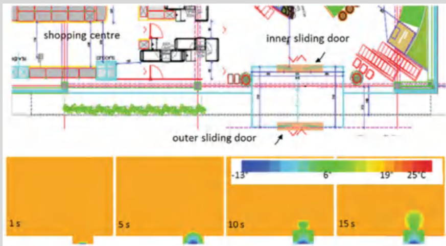
Fig. 8.4 Floor plan of entrance in shopping centre (top), air temperatures 0.15 m above the floor 1, 5, 10, and 15 s after the door is opened; calculated with PHOENICS CFD (PHOENICS, Concentration, Heat and Momentum Limited (CHAM), UK) software with the finite volume method (bottom)
