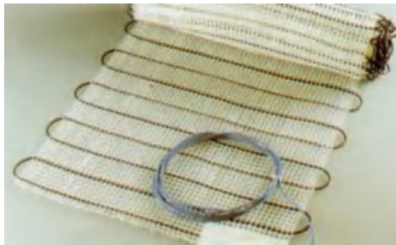
Fig. 6.6 Electric resistant heater designed to be built in the floor to prevent unpleasant “cold feet” effect if floor cover has high thermal effusivity
