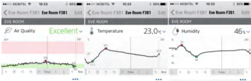
Fig. 4.2 Elgato Eve smart units include Eve Room. Devices can be used for monitoring indoor thermal comfort and IAQ. Data can be sent to actuators that can control, for example, thermostatic valves on heat emission units, fans, or lighting units (Elgato Eve, Eve Systems GmbH, 2016)
