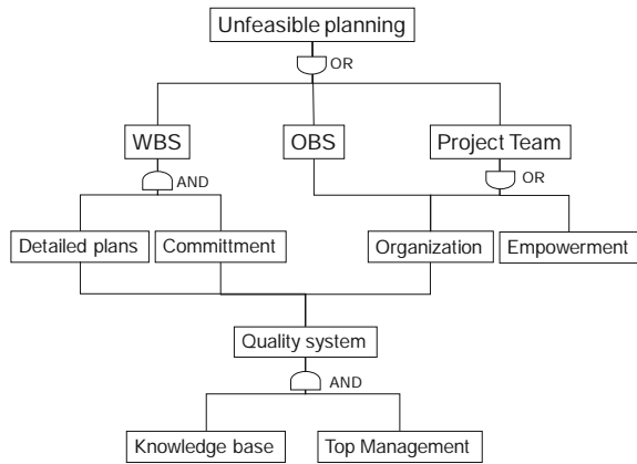
Fig. 13.1 Example of fault tree analysis
