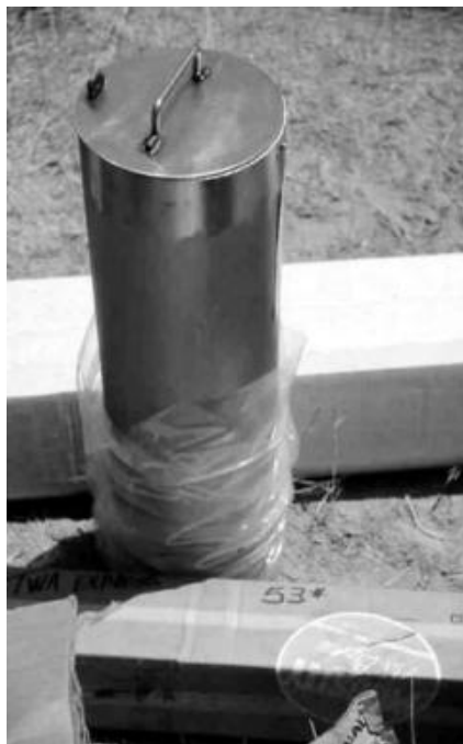
FIGURE 10.130 Stainless steel protective casing provides corrosion resistance superior to that of painted mild steel materials.
