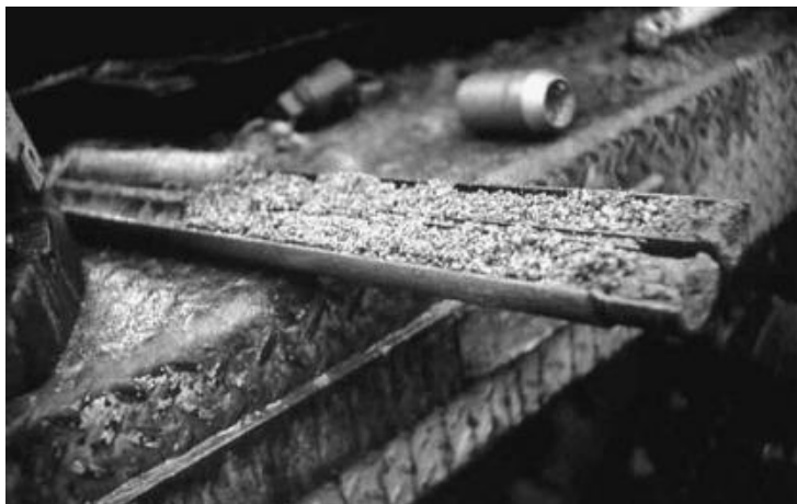
FIGURE 2.22 Standard 18 to 24 in. long, 2 in. O.D. split-spoon samplers are the most widely used soil sampling method in traditional site characterization programs. Depending on the materials sampled, recovery can range from 100% (shown here in a sand and fine gravel) to less than 15 or 20% (in dense, stiff clays or saturated fine sands).
