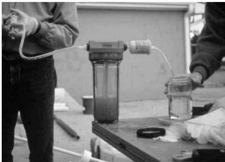
FIGURE 15.79 A positive-pressure filtration system is a better option to use for ground-water sampling. Note the removal of sediment achieved by the cartridge filter.
