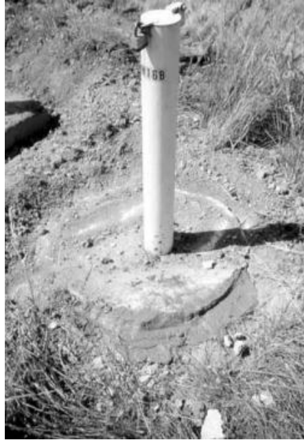
FIGURE 10.151 Monitoring well identification is usually painted or etched on the outer part of the protective well casing.
