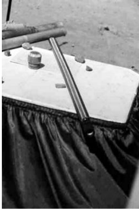
FIGURE 10.32 Prepacked well screens are viable alternatives to conventional well designs. This type of screen is routinely used in direct-push well installations.
