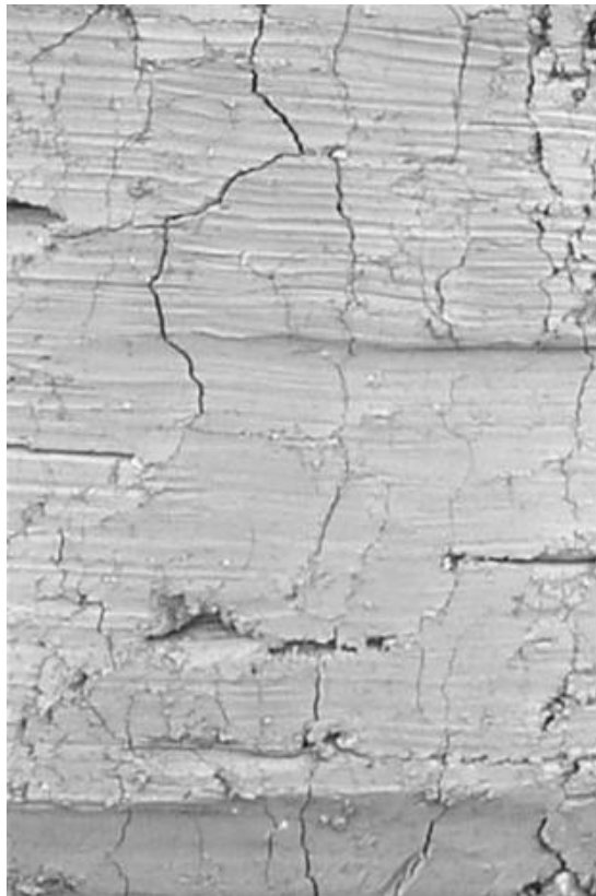
FIGURE 18.6 Clay units thought to be impermeable can behave like a porous medium if they are cracked or fractured.
