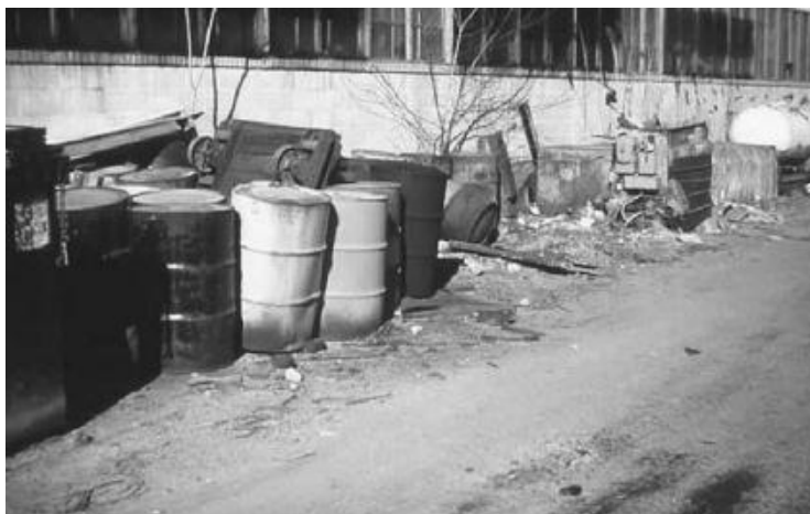
FIGURE 2.85 If site reconnaissance uncovers evidence of storage of drums of potentially hazardous materials, the field investigation should be configured to determine the contents of the drums and whether the contents have leaked into soil, surface water, or ground water.
