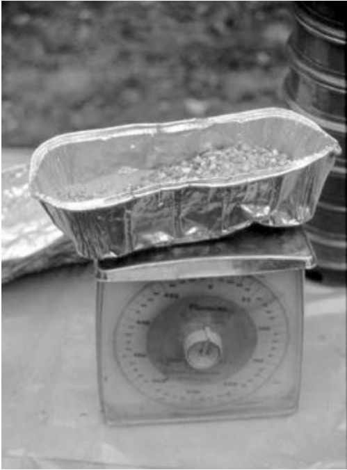
FIGURE 10.73 After the formation sample is dried, it must be weighed to obtain a total sample weight.
