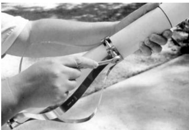
FIGURE 10.65 Attaching a bow-type centralizer to well casing using straps tightened by a bolt.
