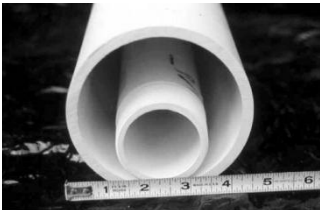
FIGURE 10.62 The diameter of a monitoring well must be selected based on a variety of factors, including volume, which may affect the amount of water that must be purged from the well. The volume of a 2-in. nominal casing (0.163 gal/ft) is \frac{1}{4} the volume of a 4-in. nominal casing (0.65 gal/ft).
