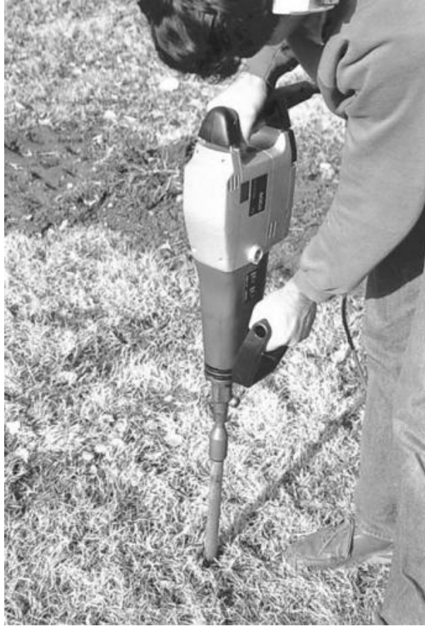
FIGURE 6.2 Several varieties of electrical or pneumatic hammers have been adapted for use in advancing DP tools. These hammers do not assist with extraction of the tools.
