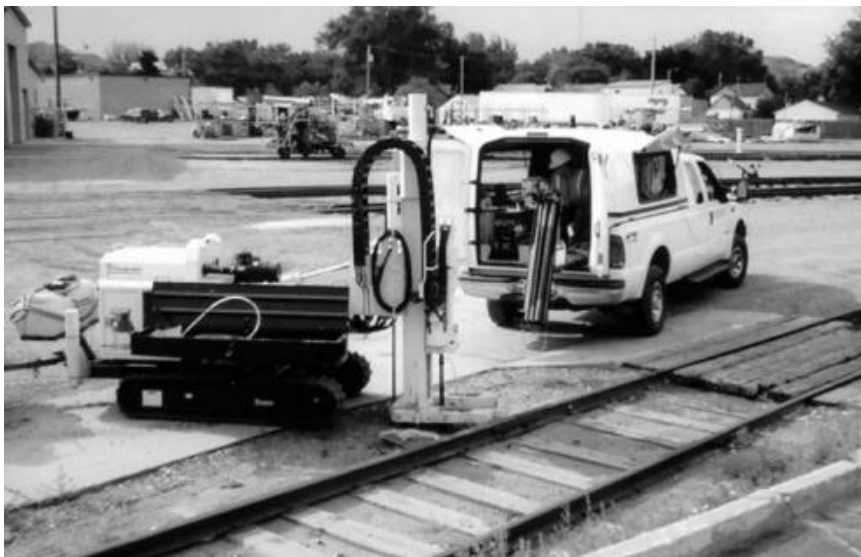
FIGURE 6.75 MIP logging operations in the field. For this project, the MIP system, including the probe rods, trunk line, and detector system, is housed in the bed of the truck shown in the background. The MIP probe is being pushed into the ground using the track-mounted DP machine in the foreground. A trunk line containing gas and electrical lines runs from the truck to the probing machine.
