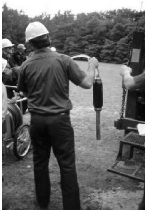
FIGURE 15.64 A packer used in conjunction with a progressing cavity pump, prior to installation.
