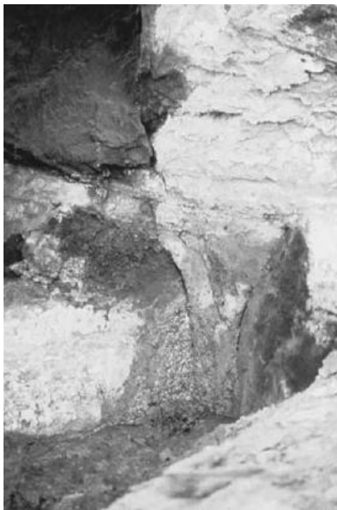
FIGURE 2.76 Leachate seeps often take the same preferential flow pathways as ground water, such as this fracture, a fact that investigators should consider when conducting site reconnaissance.
