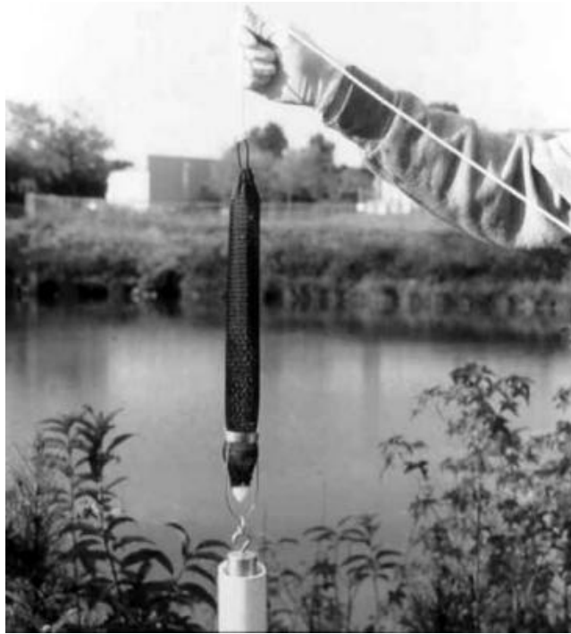
FIGURE 15.59 A PDBS prepared for deployment in a well. (Photo courtesy of Eon Products.)
