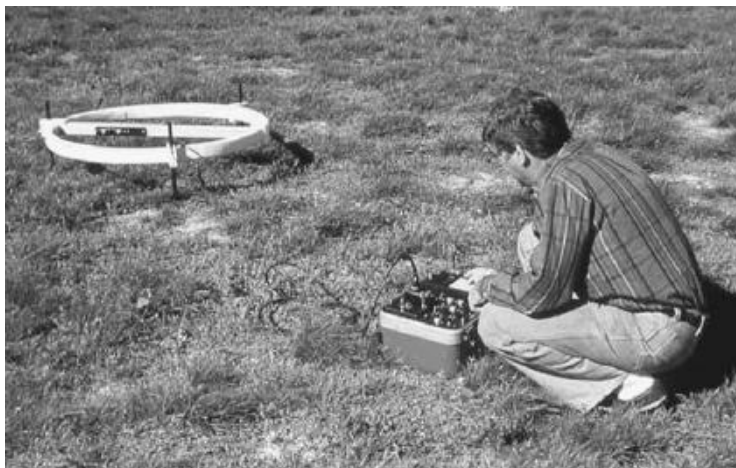
FIGURE 2.37 Real-time measurement technologies, including surface geophysics (in this case, electromagnetic conductivity), are a cornerstone of the Triad approach.
