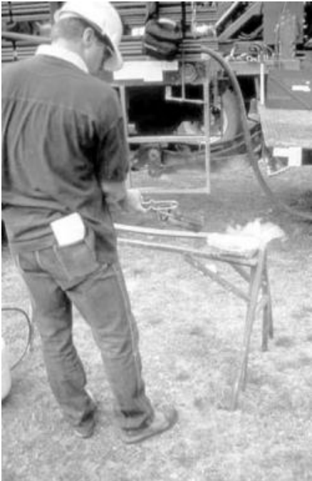
FIGURE 10.72 The first step in conducting a field sieve analysis of a formation sample is to dry the sample so it can be easily separated by running it through the sieves. In this case, the sample is being dried with a propane torch.
