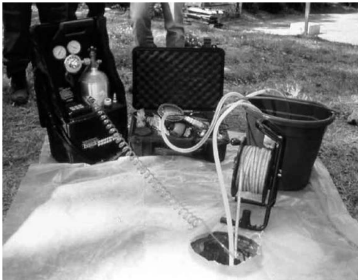
FIGURE 15.66 The equipment setup for low-flow purging and sampling includes a pump (in this case, a dedicated bladder pump); a pump controller with drive gas (left); a flow-through cell (center) with sensors for measuring pH, temperature, specific conductance, DO and ORP, and a water-level gauge (right) for measuring drawdown during pumping.
