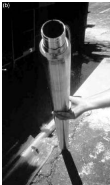
FIGURE 10.101 This prepacked well screen consists of two concentric well screens welded together, with filter-pack sand installed in between. Small-diameter versions are also widely used in direct-push well installations.
