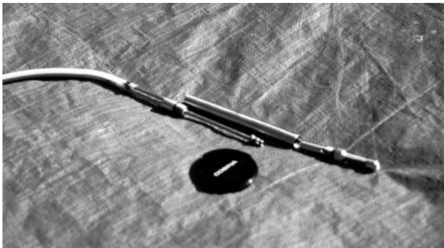
FIGURE 6.58 A small-diameter gas-drive pump, disassembled for cleaning.
