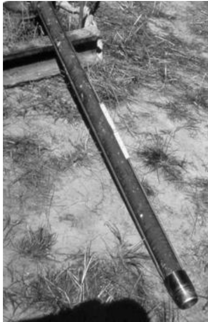
FIGURE 5.11 Continuous tube sampler (used with hollow-stem auger).
