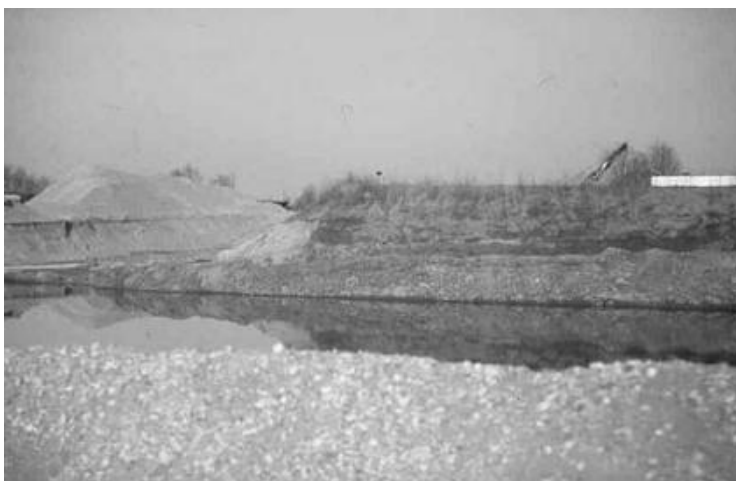
FIGURE 2.97 Man-made excavations, such as this sand and gravel operation, provide excellent opportunities to gain insight into shallow regional and local geology. The character of geologic materials in this gravel pit (adjacent to the site being investigated) confirmed information on regional geologic maps and allowed investigators to get a first-hand view of the depth to ground water.
