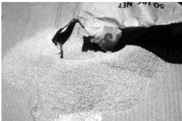
FIGURE 10.84 Filter-pack material should be composed of clean quartz sand (less than 5% nonsiliceous material).
