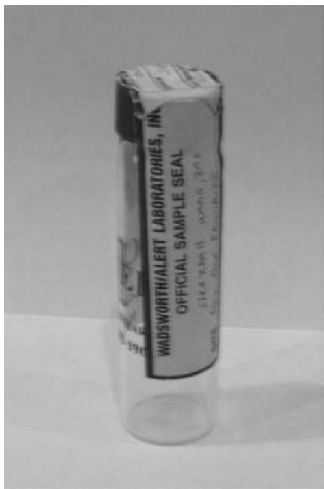
FIGURE 15.96 If the sample seal on a VOC vial covers the septum, the constituents of the adhesive from the seal may be detected in the analysis as the needle from the analytical instrument penetrates the septum to collect the sample.
