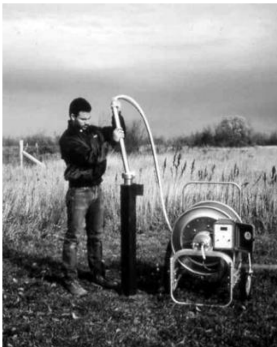
FIGURE 15.54 A progressing cavity pump is a relatively portable pump that operates on 12 V DC power supplied by a deep-cycle marine battery.
