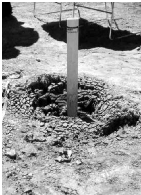
FIGURE 10.111 Bentonite grouts are not suitable for use at the surface in arid climates.
