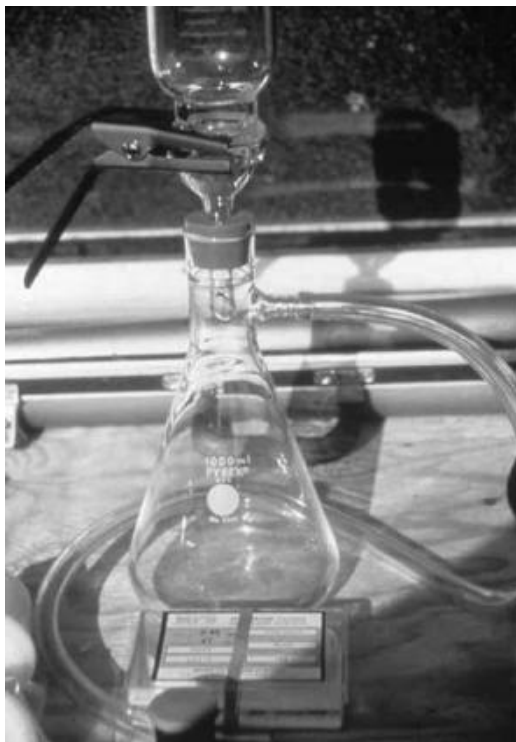
FIGURE 15.78 A vacuum filtration system used for ground-water sampling. This practice is not encouraged.
