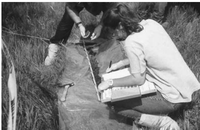
FIGURE 2.23 Samples or portions of a sample not destined for lab analysis are examined in the field to determine physical characteristics, using one of several available soil classification systems and a standard set of sample descriptors including color, moisture content, organic matter content, and other descriptors as noted in Table 2.1.
