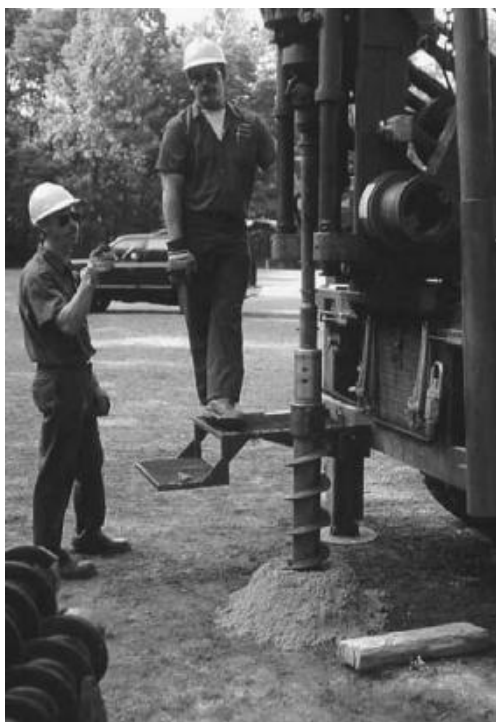
FIGURE 2.115 The hollow-stem auger is the most commonly used conventional drilling method for conducting environmental field work. However, augers are unable to penetrate bedrock, boulders, or gravel and cobble zones, and they produce significant amounts of IDW.
