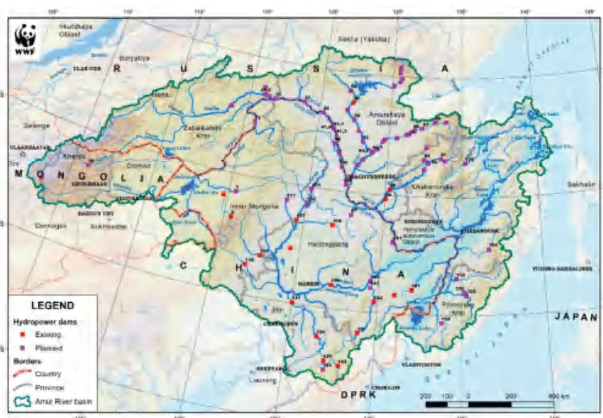
Figure 2. Locations of the existing and potential dams in the Amur River basin. © WWF-Russia.
