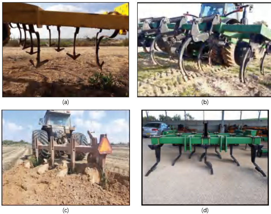
Figure 2. Tillage tools used during the experiment: (a) Sweep-knives (SK) cultivator; (b) Chisel-knives (CK) cultivator; (c) Plow; (d) Subsoiler (paraplow type).
