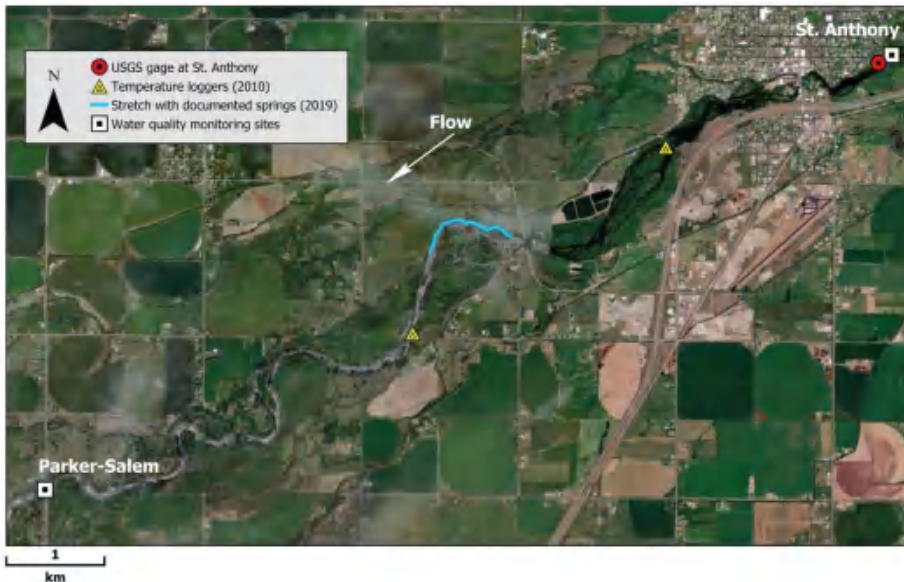
Figure 2. Map of field study reach, showing locations of U.S. Geological Survey (USGS) streamflow gage at St. Anthony, temperature loggers deployed in 2010, water-quality monitoring locations, and stretch where springs were documented in 2019. Data credit: ESRI.
