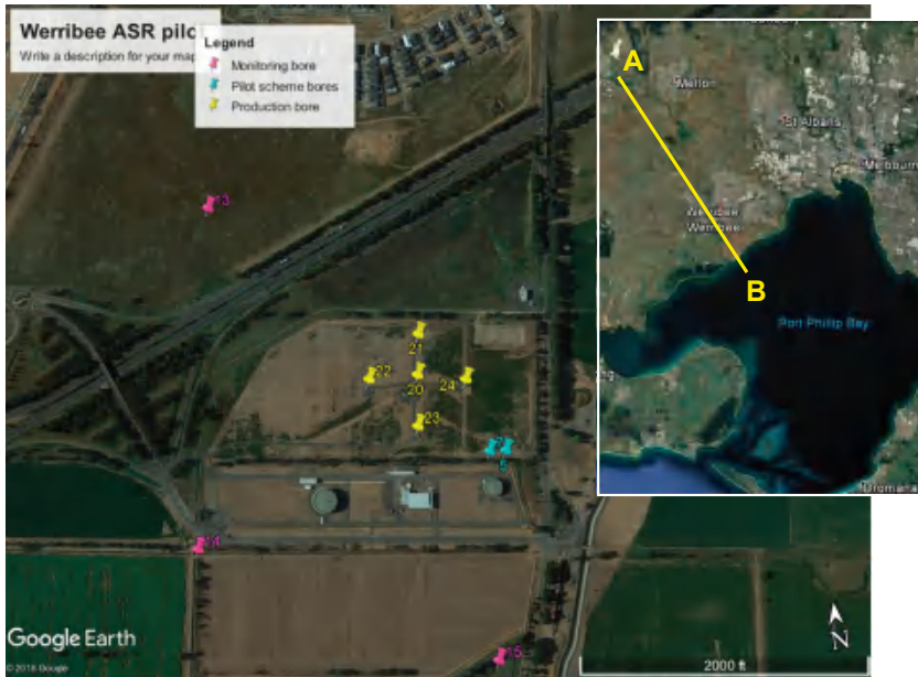
Figure 1. Site map showing the location of the aquifer storage recovery (ASR) (production) and monitoring wells. ASR well 5 was the production well during the trial in 2012, with its monitoring well 7 at ca. 40 m distance. Production wells 20–24 form together the future West Werribee ASR plant, but for now they are part of the second pilot, with well 20 as ASR well and 21–24 as monitoring wells. AB = geological section shown in Figure 2.
