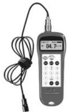
FIGURE 7.15 Sonic tension meter tensioning.
