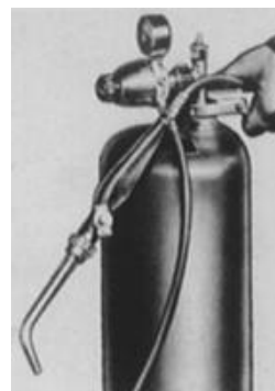
FIGURE 2.2 Connecting a typical air-acetylene outfit. The standard type of portable outfit is shown. Smaller tanks also are available.
