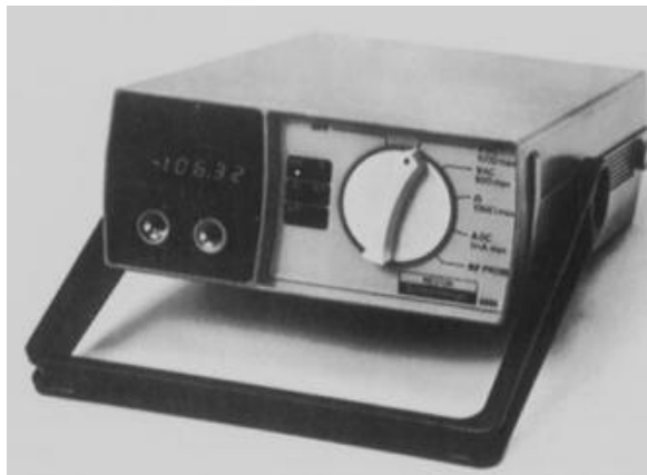
FIGURE 2.6 Four-digit autoranging DMM. (Weston Instruments, Inc.)
