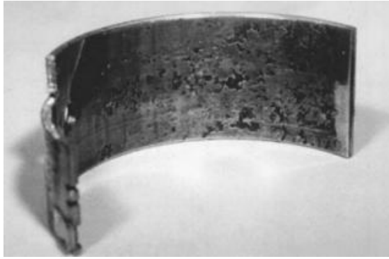
FIGURE 1.10 Fatigue of bearing lining.
