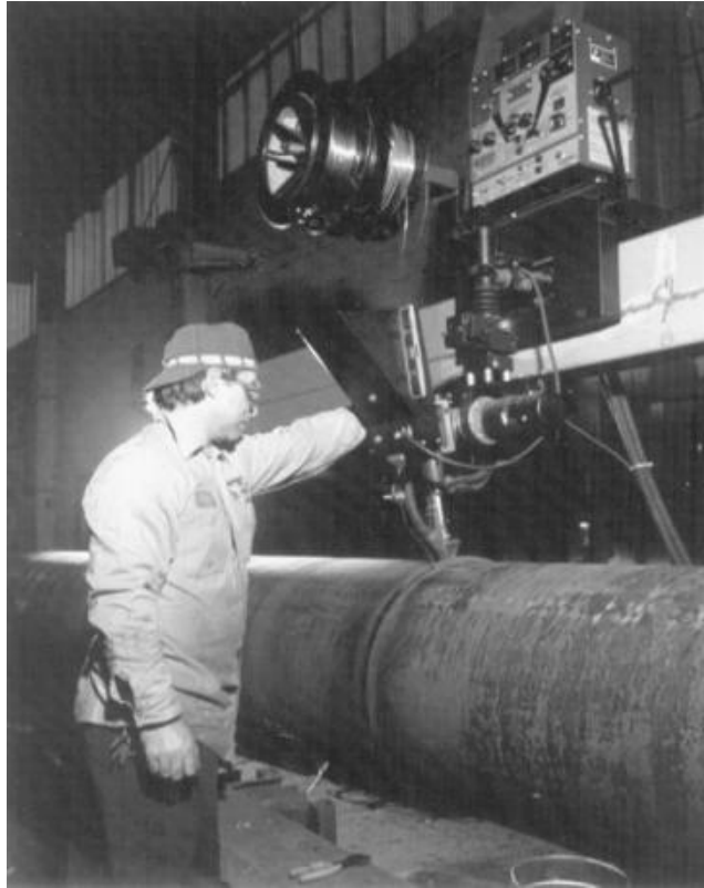
FIGURE 1.34 Fully automatic welding equipment.
