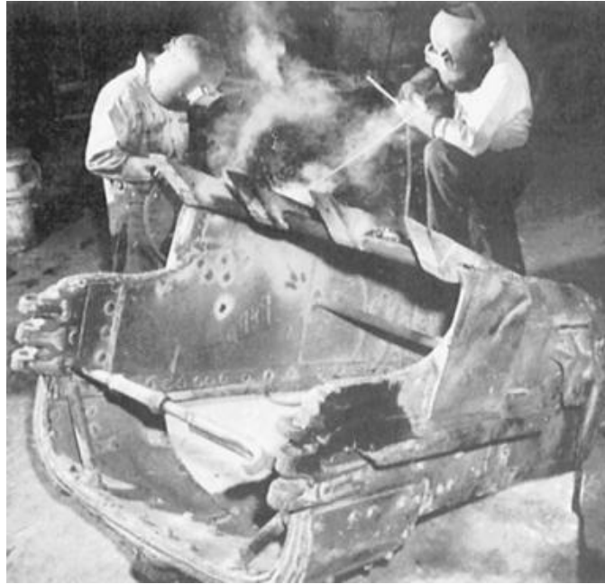
FIGURE 1.35 Shielded metal arc welding is used to rebuild and to hard-surface worn areas of a dragline bucket.
