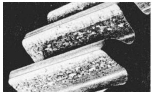
FIGURE 8.5 Severe pitting caused by overloading gear.
