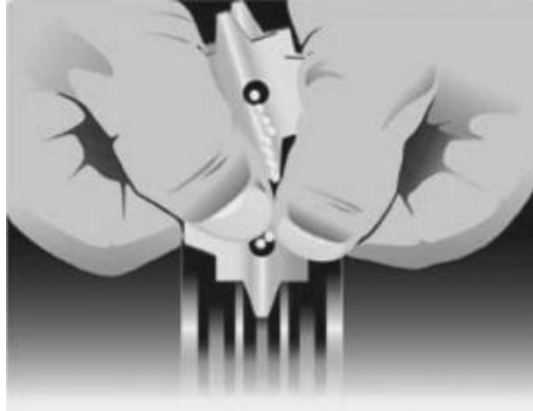
FIGURE 7.10 Sheave groove inspection.
