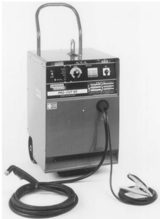
FIGURE 1.30 Power source for plasma arc cutting.
