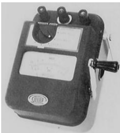
FIGURE 2.26 Portable megger. (James G. Biddle Company.)
