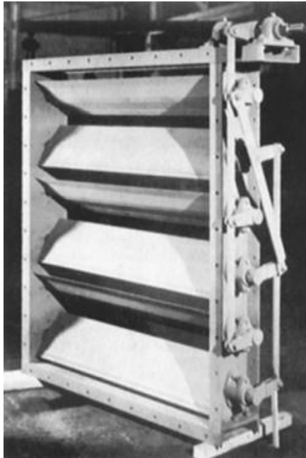
FIGURE 6.12 Outlet damper with streamlined blades and linkage arranged to move adjacent blades in opposite directions for even throttling.
