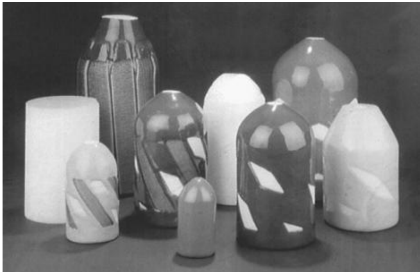
FIGURE 2.8 Specialized foam pigs are available for almost every pipeline cleaning requirement, from light cleanings, wiping, and drying (squeegeeing), to heavy buildup removal and scraping. Pigs can be used in lines of less than 2 in. diameter to 144 in. (12 ft) diameter. These various pigs have a concave base and conical head design to increase speed and effectiveness, and the spiral/crisscross bands of abrasive material create a patented rotating motion, further enhancing cleaning. ( Courtesy of Girard Industries, Inc., Houston, Tex. )
