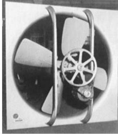
FIGURE 6.8 Belt-driven propeller fan for medium duty. Most units can be obtained for air-flow in either direction. This fan is for wall mounting and will exhaust air from a space, drawing it over the motor and the drive.
