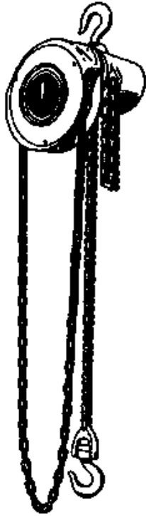
FIGURE 6.3 Spur-gear single-reeved hoist with roller chain.
