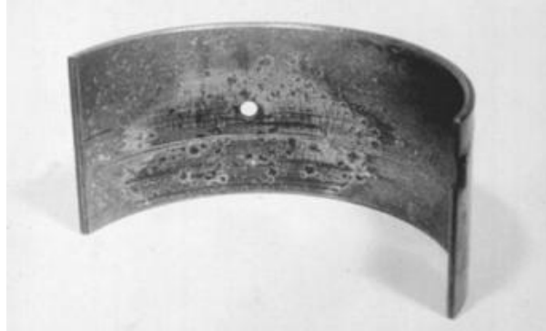
FIGURE 1.8 Bearing with severe dirt embedment.
