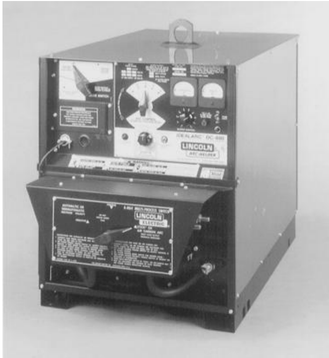
FIGURE 1.46 Motor-generator with rectifier.
