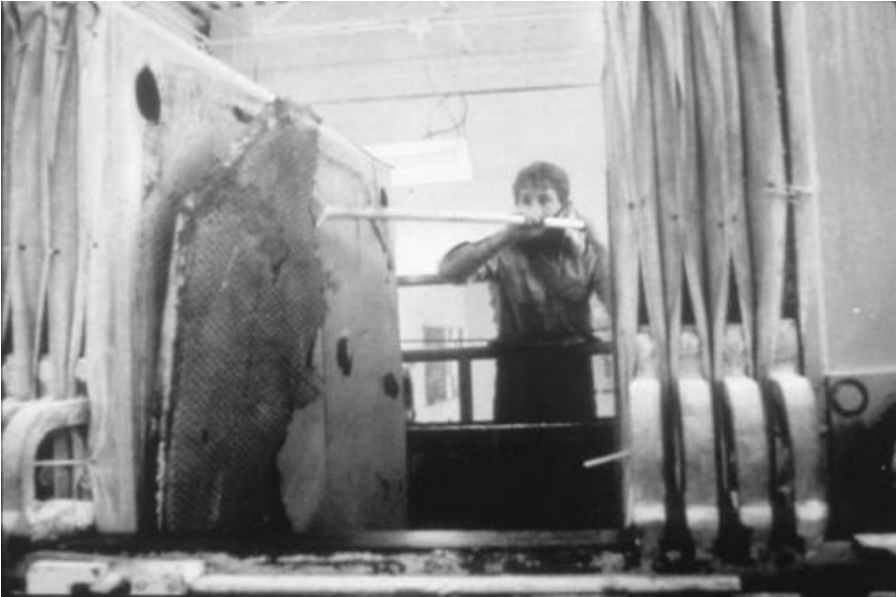
Fig. 23–22. Typical method for dewatered cake removal from filter press
