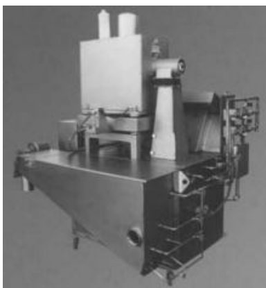
Fig. 24-19. (a) Photo of paste-type lime slaker (Courtesy of USFilter/Wallace and Tiernan); (b) Photo of detention-type slaker (Courtesy of Penn Process/Omega)
