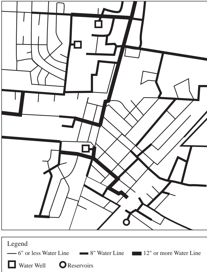
Fig. 7-3. Example of a water system map
