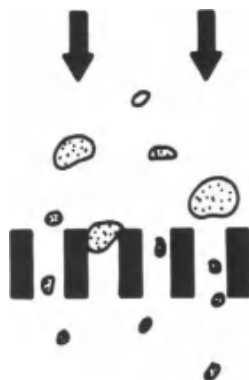
Figure 1.1. Filtration by surface straining 21 .
