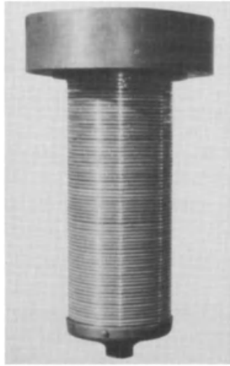
Figure 9.31. A multi-segment stack assembly for polymer filtration.
