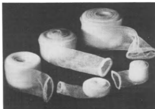
Figure 6.11. Examples of stocking or double-layered knitted mesh.
