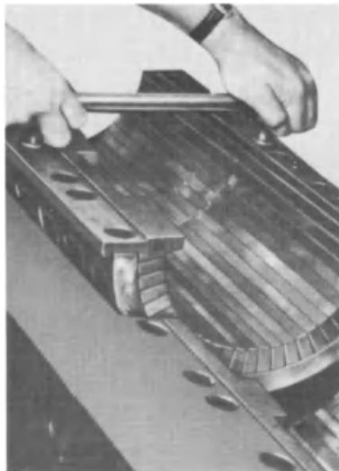
Figure 6.30. Assembling the bar screen cage of a high pressure screw press. (Photograph: The French Oil Mill Machinery).
