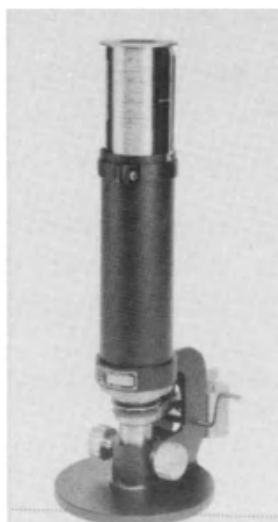
Figure 11.2. Gurley Densometer for measuring air permeability.
