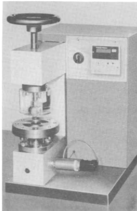
Figure 11.26. A digital bursting strength tester with manual clamping.
