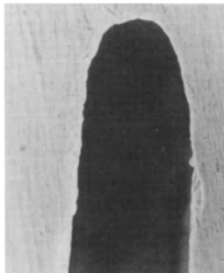
Figure 6.21. High magnification ( \times 720 ) of SSL slot after 1350 h operation. (Photograph: Laser Action Pty Ltd)
