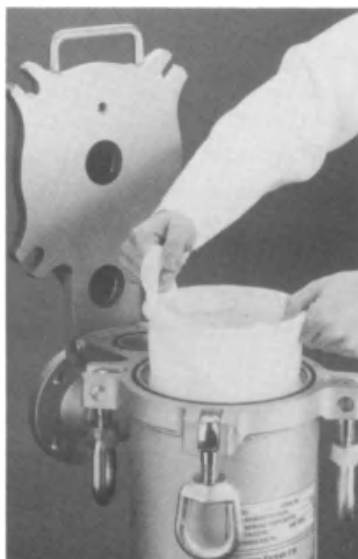
Figure 9.6. Fitting a bag filter into an enclosed housing.
