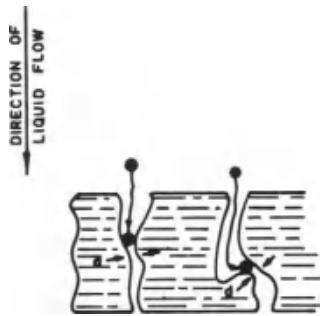
Figure 1.2. Filtration by depth straining 31 .
