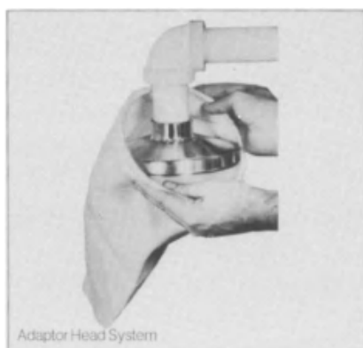
Figure 9.5. Fitting a bag filter to an adaptor head for open filtration.
