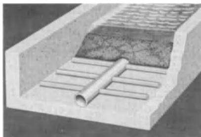
Figure 6.28. Johnson channel rod underdrain for sand filter.
