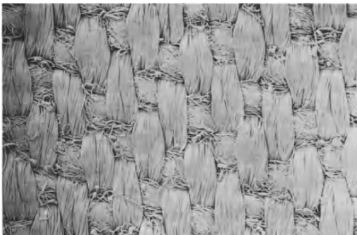
Figure 2.8. A mixed yarn reverse-satin weave fabric, with multifilament warp and staple weft.
