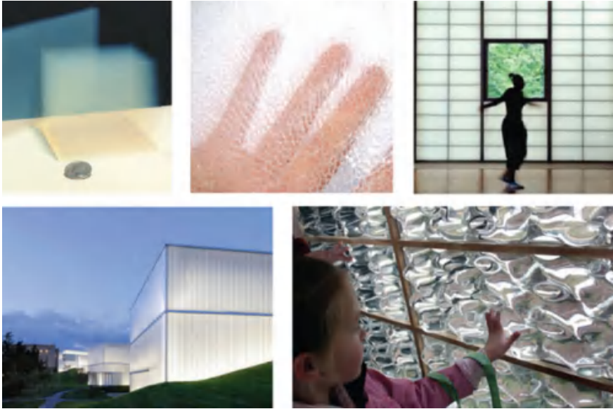
Fig. 4.26 Transparent insulation examples (Happold 2016)
