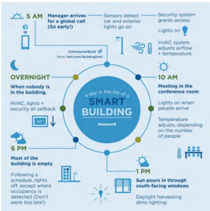
Fig. 6.5 An illustration of how smart building applications can take automatic actions to optimize energy costs and occupant comfort (Source Honeywell)
