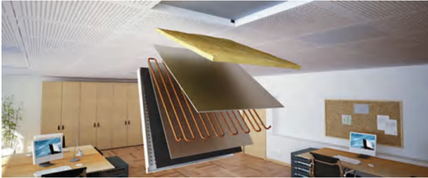
Fig. 5.7 Chilled ceiling panel components (SGL Carbon 2012)
