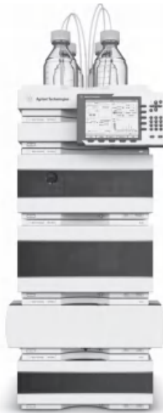
FIGURE 17.3 High-performance liquid chromatography unit. (Photo courtesy of Agilent Technologies, Inc., Santa Clara, CA.)
