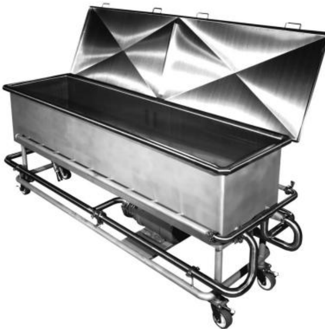
FIGURE 12.9 Typical COP station. (Courtesy of Electrol Specialties Company (ESC), South Beloit, IL.)
