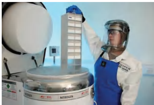
FIGURE 12.25 Cell bank being lifted out of a liquid nitrogen freezer. (Courtesy of FUJIFILM Diosynth Biotechnologies, Morrisville, NC.)
