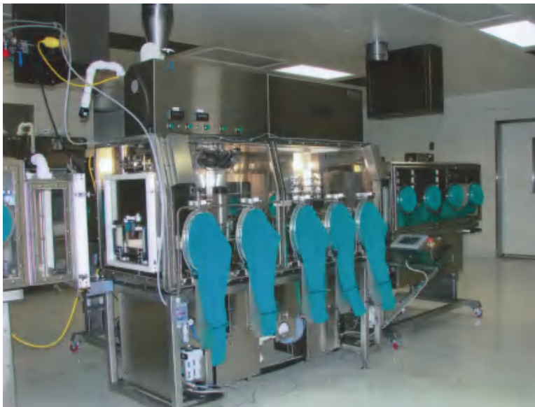
FIGURE 14.3 Aseptic filler isolator with docking. (Courtesy of Schaefer Technologies, Indianapolis, IN.)
