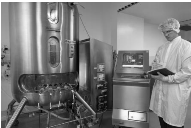
FIGURE 12.13 Aseptic closed processing with single-use or disposable technology. (Courtesy of FUJIFILM Diosynth Biotechnologies, Morrisville, NC.)
