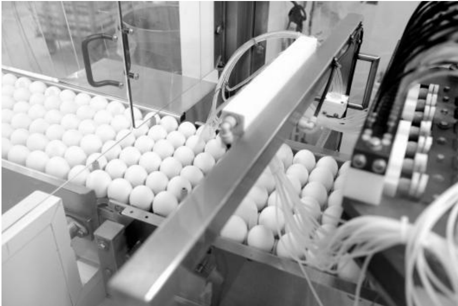
FIGURE 12.5 Flu vaccine production: eggs being inoculated with the seed virus (Val de Reuil, France, March 2009). (Courtesy of Vincent Moncorgé; copyright Sano Pasteur, Lyon, France.)
