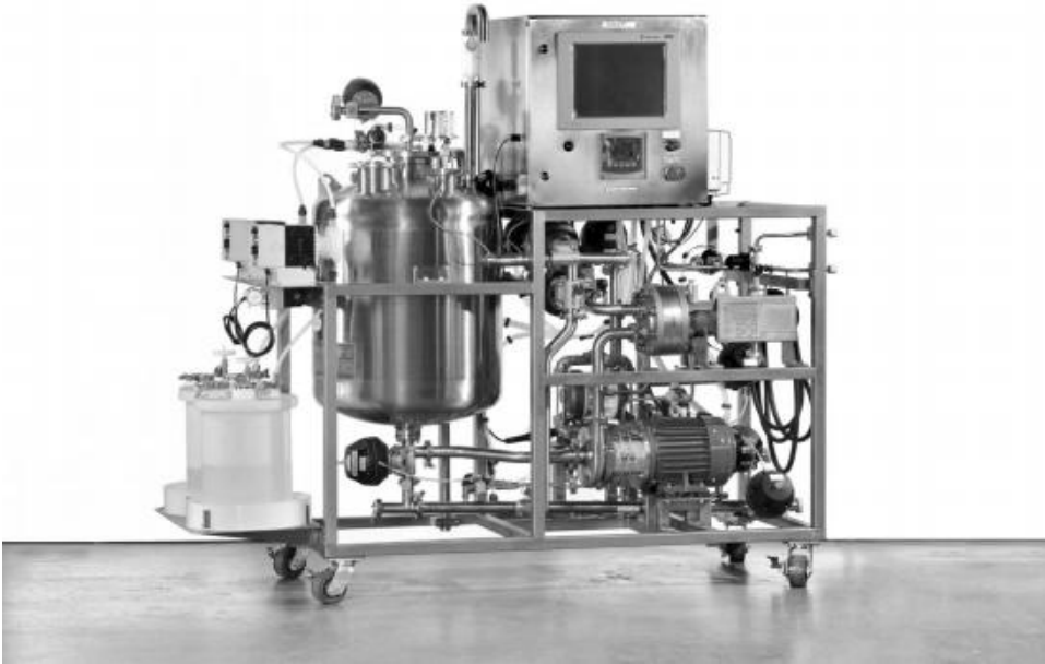
FIGURE 12.8 Portable CIP station. (Courtesy of ABEC, Bethlehem, PA.)
