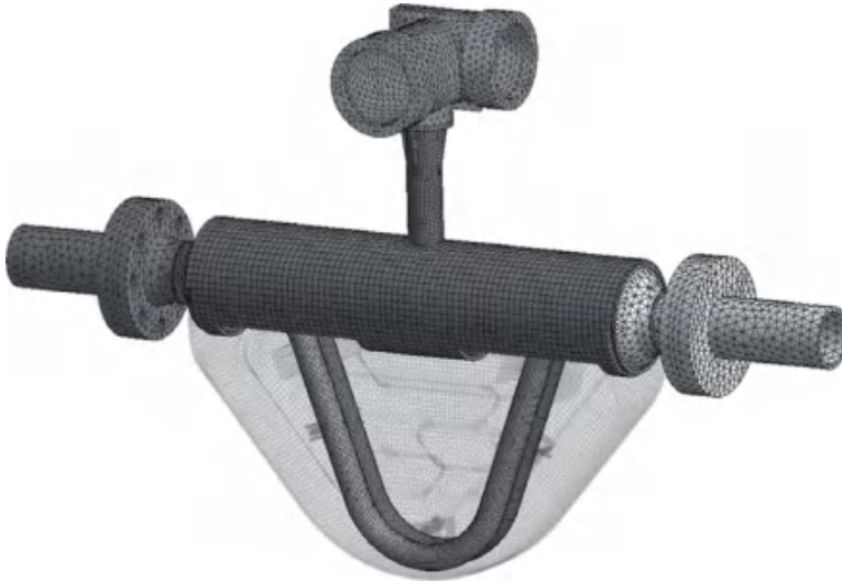
Figure 20.A.4. A typical finite element (FE) model for a complete Coriolis flowmeter (KROHNE's latest generation of twin bent-tube flowmeters) together with adjacent process connection and pipes (Reproduced with the kind permission of KROHNE).
