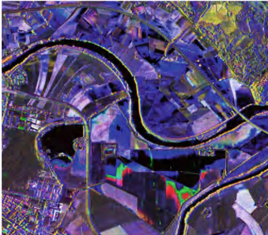
Fig. 18 RGB composition of three COSMO-SkyMed intensity images of the 2009 Alessandria (Italy) flood. Red April 29, 2009, green April 30, 2009, blue May 1, 2009 (From Pulvirenti et al. [45], © 2010 Elsevier Inc. All rights reserved)
