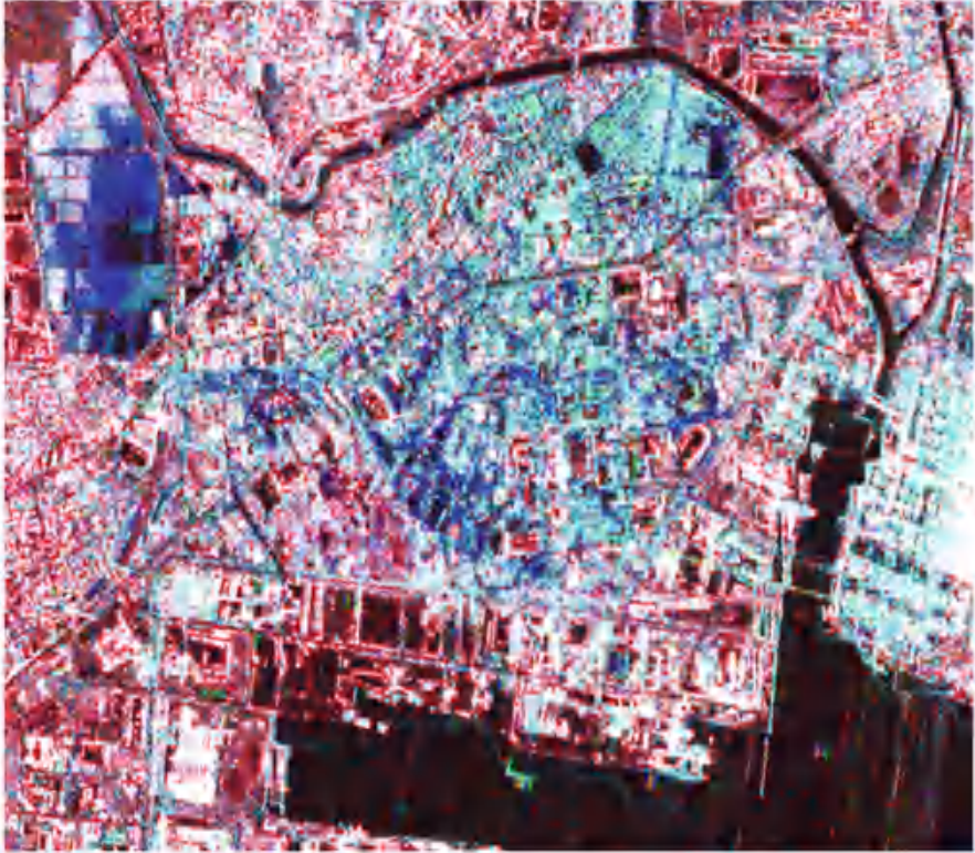
Fig. 21 RGB color composite images of the Sendai harbor created by using the COSMO-SkyMed observations of the 2011 Japan tsunami acquired on March 12 and March 13, 2011. Red coherence between the two images, green March 12 intensity, blue March 13 intensity (From Chini et al. [10], © 2012 IEEE)
