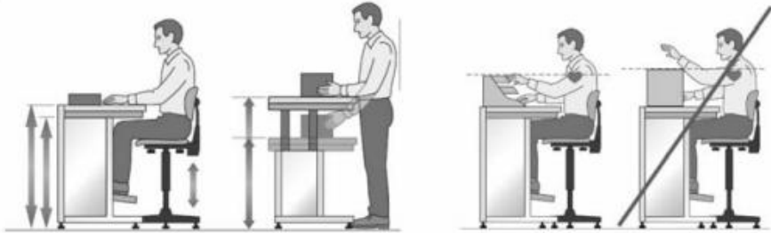
Fig. 5.21 Heart height and working position
