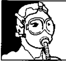
FIGURE 17.17 Illustration of full facepiece respirator.
