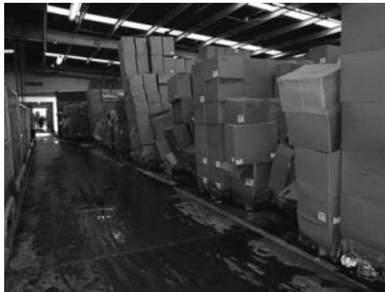
FIGURE 7.8 If Lower Boxes in a Distribution Warehouse Are Exposed to Water, the Stacks Become Unstable.
