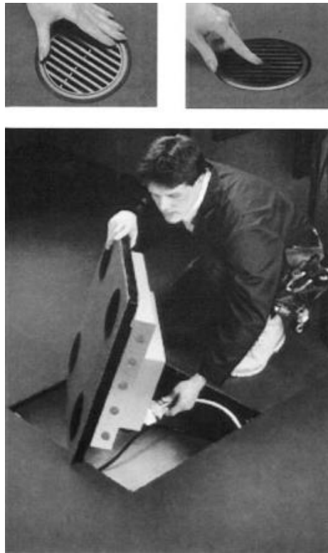
FIGURE 12.11b Tate Task Air Module™—Four Independent Grills Rotate a Full 360° for Complete Control of Air Direction. An Easy-to-Use Thumbwheel Fan Speed Control Provides Adjustment of Air Volume from Off, to Low, Medium, and High Speeds. Quick Connect/Disconnect Electrical Connectors Make Installation of a Task Air Module™ Easy and Simple (Courtesy: Tate, Inc.).
