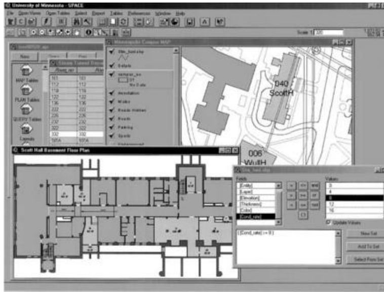
FIGURE 30.8 New CMMS Integrated with the SPACE System.
