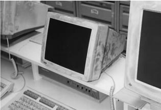
FIGURE 7.3 After the World Trade Center Explosion, Electronic Equipment on All Floors Required Restoration.
