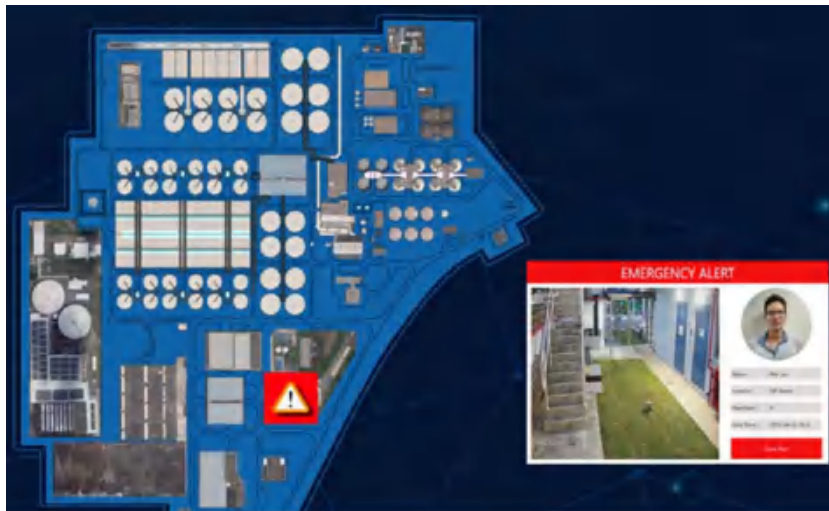
Figure 3.10 Geo-fencing intruder alert system.
