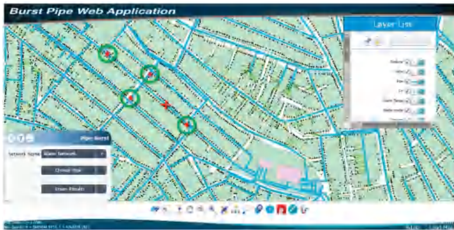
Figure 4. Interface, view of the area around damaged pipe and valves linked to damaged pipeline.
