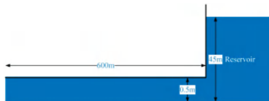
Figure 17. A sketch of the conduct-reservoir model.
