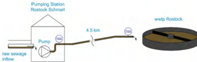
Figure 1. Schematic view of the study side. Total suspended solids (TSS) are measured inside the pressure pipe in pumping station (PS) Rostock-Schmarl and at the outflow side in the wastewater treatment plant (wwtp) Rostock after 4.5 km.
