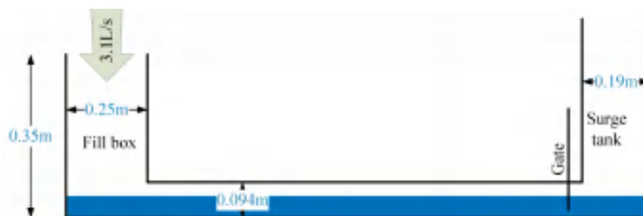
Figure 20. A sketch of the experimental setup.
