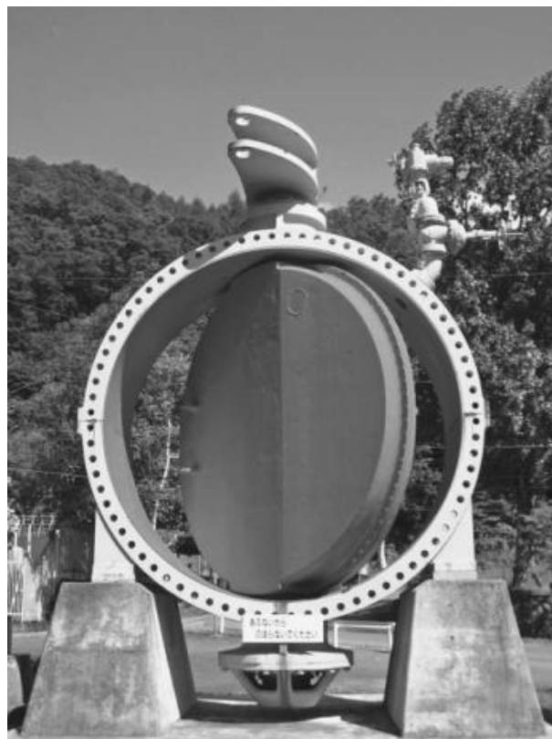
Figure 6.7 Internals of a large butterfly valve (Source: http://upload.wikimedia.org/wikipedia/commons/d/d5/Yagisawa_power_station_inlet_valve.jpg ).
